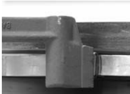
Figure 2-19: BAND-IT® Tool Bending over Retaining Clip
