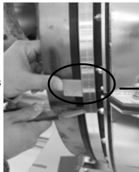
Figure 2-24: Splice Protector Plate Installation
