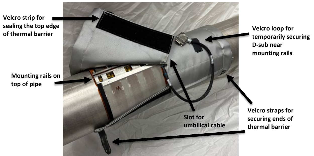
Figure 2-13: Thermal Barrier Installation over BAND - 6" to 30"
