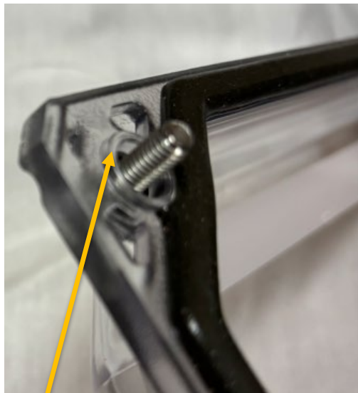
Molded-in shoulder around cover screw at corners of hinged transparent door of TRANSMITTER enclosure
