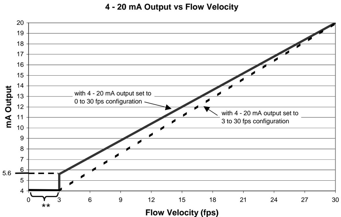
At the system Low Flow Cut Off of 3.0 fps, the value from the 4 – 20 mA output will be 5.6 mA.
