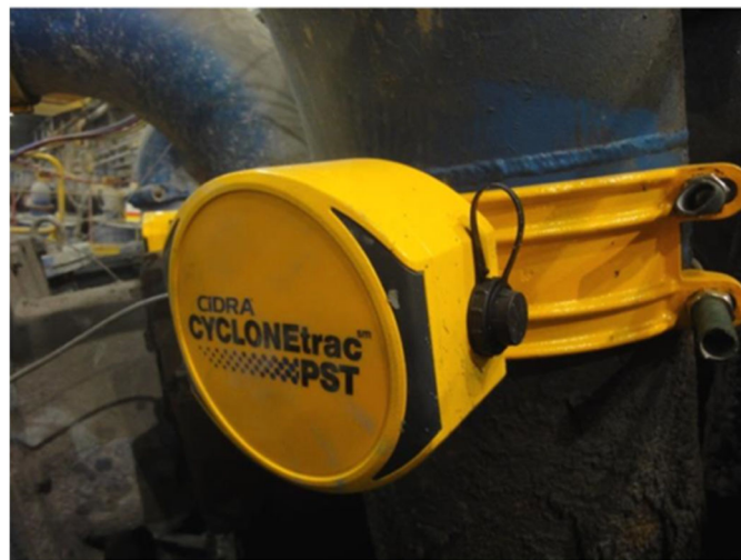
Figure 1. CYCLONetrac PST particle sizing sensor mounted on hydrocyclone overflow pipe.
