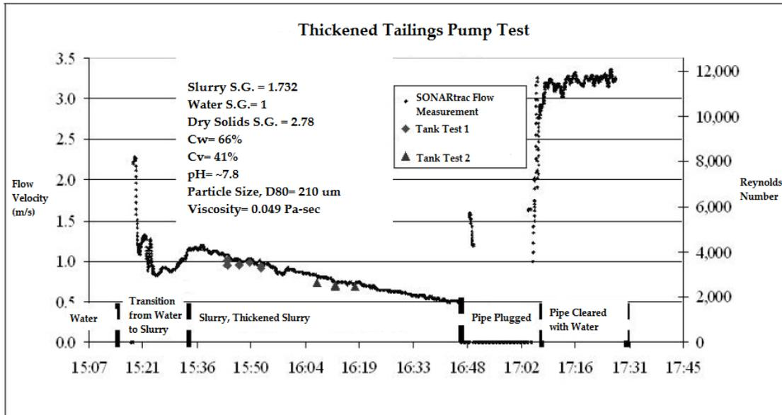
Figure 9 Thickened Tailings Flow Measurement
