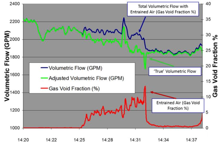
Figure 1: Gas void fraction and adjusted volumetric flow
