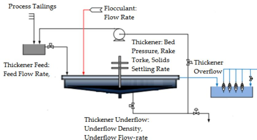
**Figure 3** Common thickener configuration with independent and dependent variables
