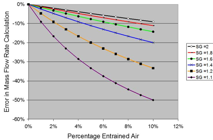
Figure 2: Entrained air measurement used to correct density measurement errors
