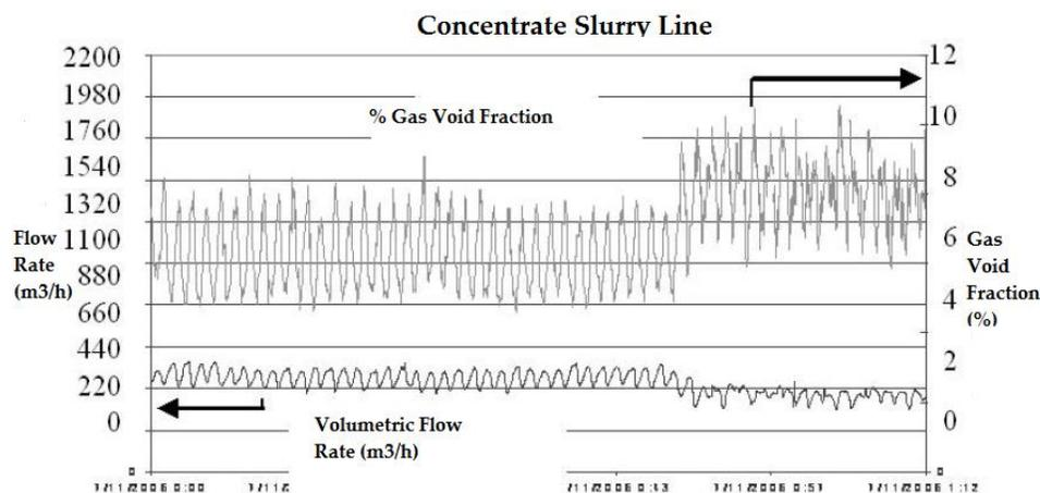
**Figure 7** Relationship between Gas Void Fraction and Volumetric Flow Rate
