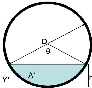
**Figure 5:** Variables in Partially Full Pipe
