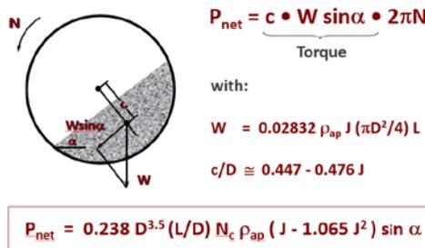
**Figure 2** Hogg & Furstenau Model for Mill Power Draw
