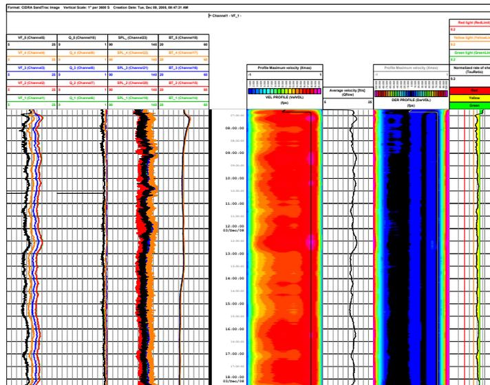
Figure 6: Hydrotransport line results, warning conditions
