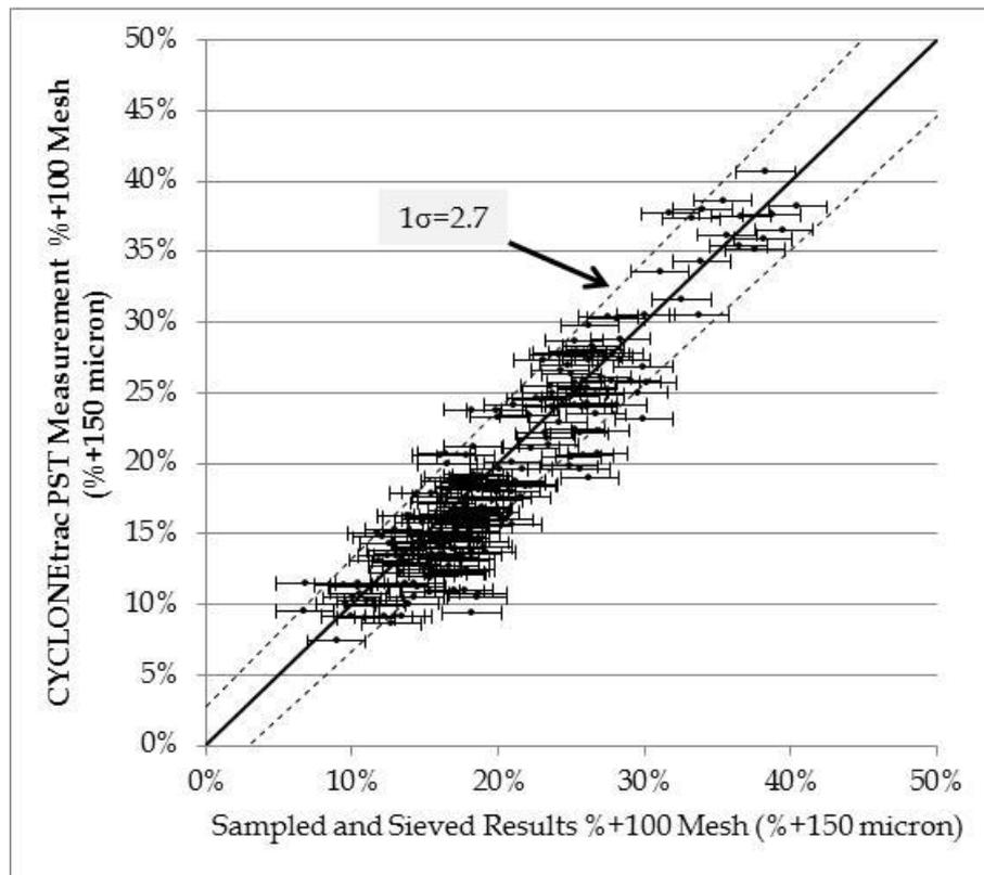
Figure 3. Comparison of CYCLONetrac PST measurement with sampled and sieved data from a major copper concentrator. Dashed lines indicate calculated one standard deviation of 2.7.
