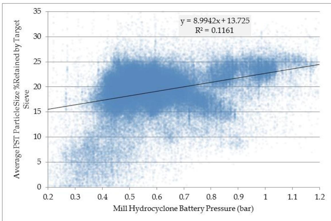
Figure 8. Cross-plot of particle size as averaged from operating cyclones versus cyclone battery pressure.
