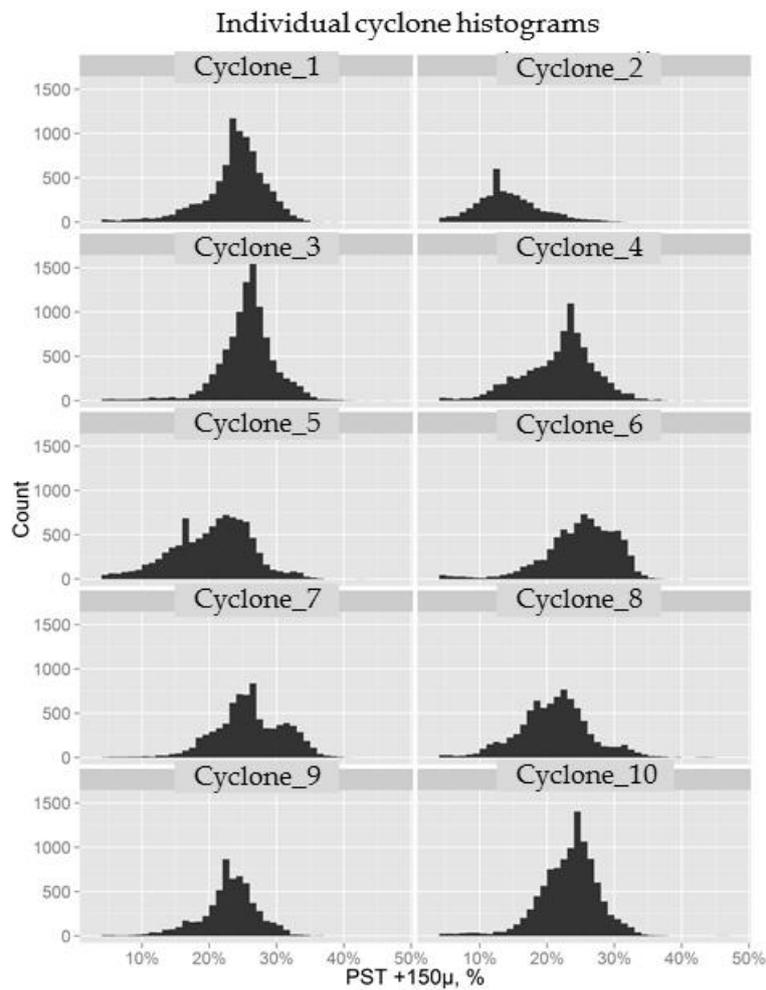
Figure 5. Histograms of particle sizes from the 10 cyclones on a battery over a one-month period.
