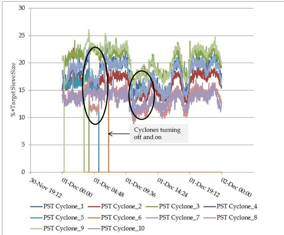
Figure 7. Time trace of particle size measurements on different cyclones on same battery indicating static and dynamic differences.
