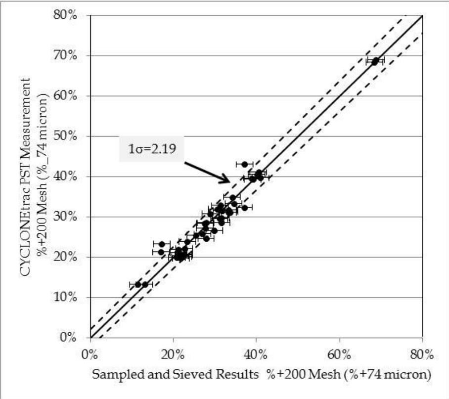
Figure 4. Comparison of CYCLONEtrac PST measurement with sampled and sieved data from copper, gold, and silver concentrator. Dashed lines indicate calculated one standard deviation of 2.17.
