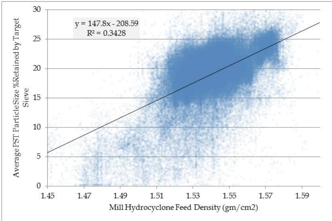
Figure 9. Cross-plot of average cyclone overflow particle size versus cyclone battery feed density.
