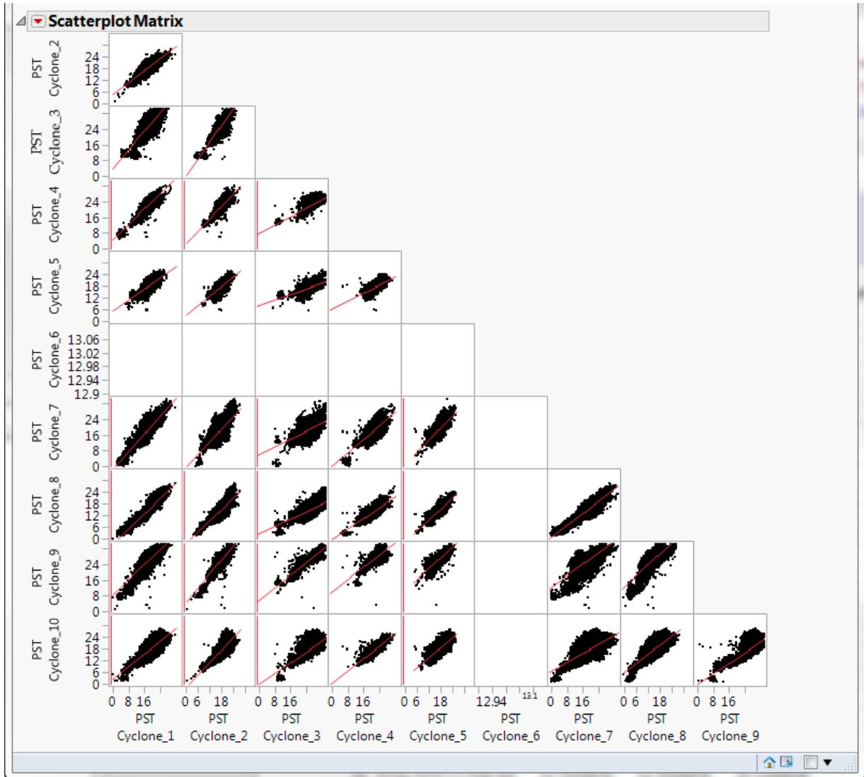
Figure 6. Scatterplots of particle size measurements from CYCLONETRAC PST on individual cyclones.
