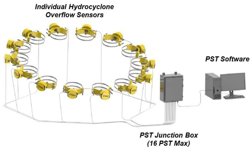
Figure 2. Illustration of particle sizing system.
