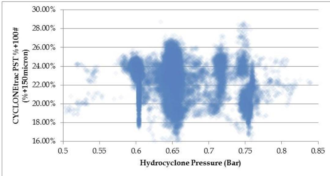
Figure 10. Particle size retained by 100 mesh screen as measured with CYCLONETrac PST versus hydrocyclone battery pressure at mine site no. 1.
