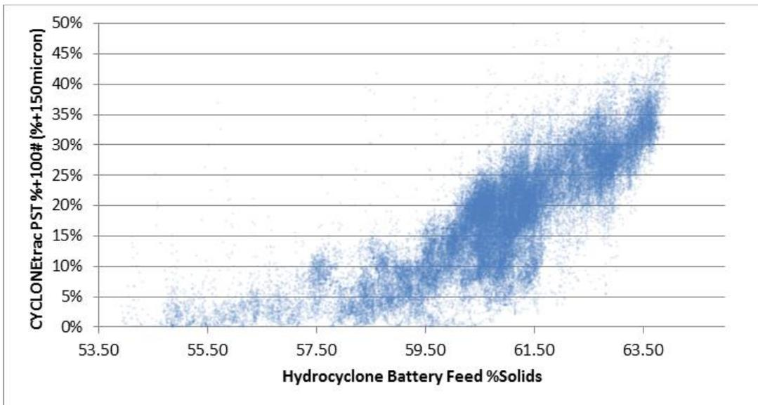
Figure 13. Particle size retained by 100 mesh as measured with CYCLONETrac PST versus % solids in the feed to the hydrocyclone battery at mine site no. 2.
