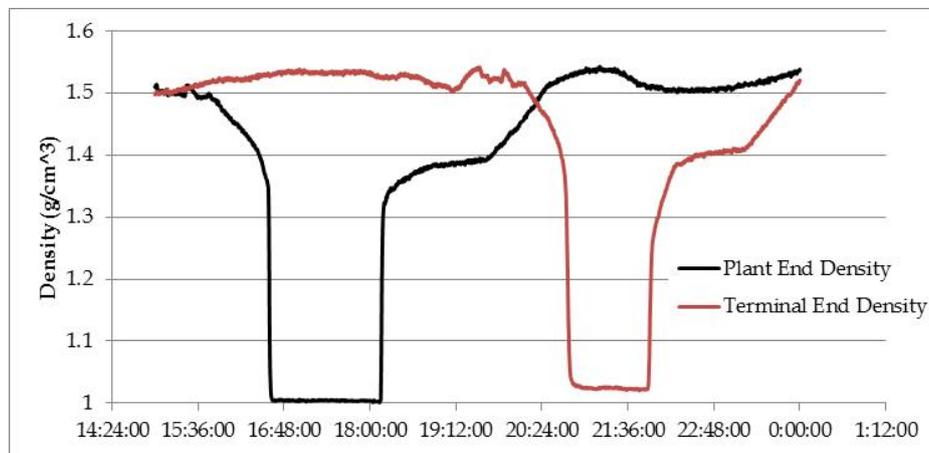
Figure 4. Density readings from nuclear density gauges at the two ends of a 50 km pipeline, showing water slug passing from the plant end to the terminal end.
