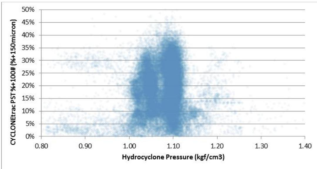
Figure 11. Particle size retained by 100 mesh screen as measured with CYCLONETrac PST versus hydrocyclone battery pressure at mine site no. 2.
