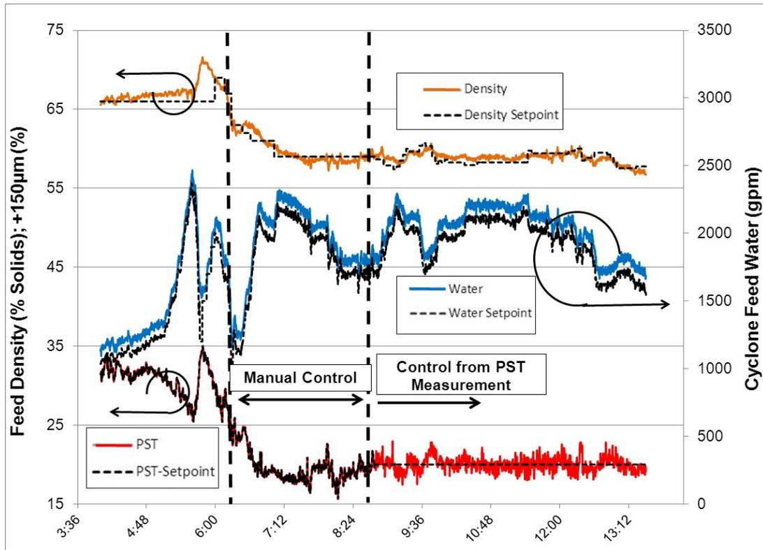
Figure 16. Manipulating density for CYCLONEtrac PST control.
