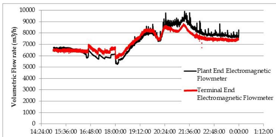
Figure 6. Electromagnetic flow meter readings of volumetric flow with varying density.
