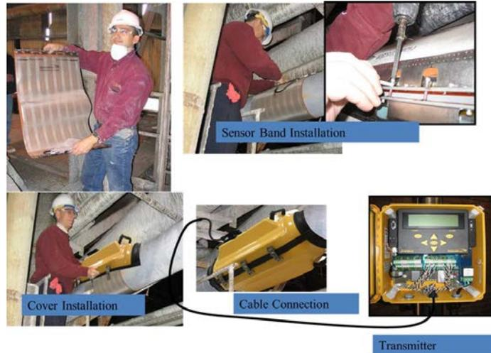
Figure 2. One implementation of array-based flow meter.
