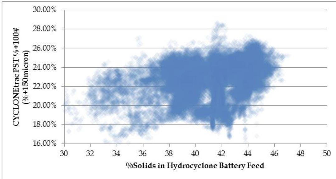
Figure 12. Particle size retained by 100 mesh screen as measured with CYCLONETrac PST versus % solids in the feed to the hydrocyclone battery at mine site no. 1.
