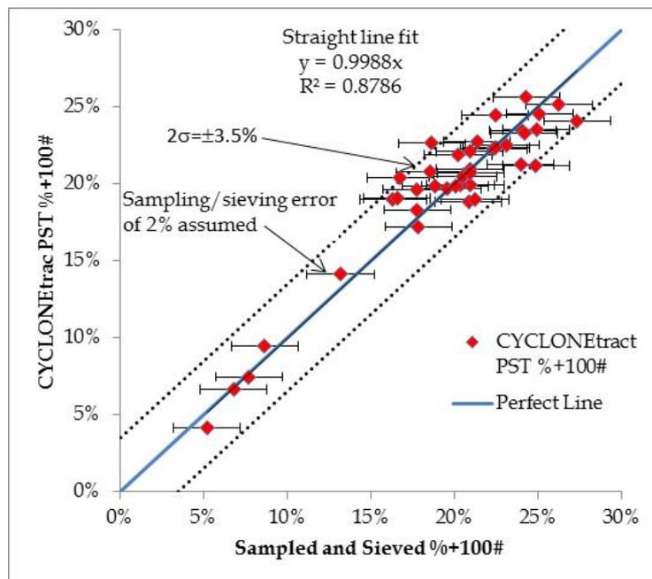
Figure 9. Example of PST results from a single cyclone compared to sampled and sieved measurements.
