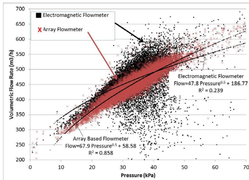
Figure 3. Hydrocyclone feed line electromagnetic flow meter (black squares) and array-based flow meter (red X) compared to pressure.
