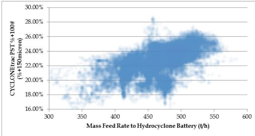
Figure 14. Particle size in the hydrocyclone overflow as a function of the mass flow rate of solids fed to the hydrocyclone battery at mine site no. 1.
