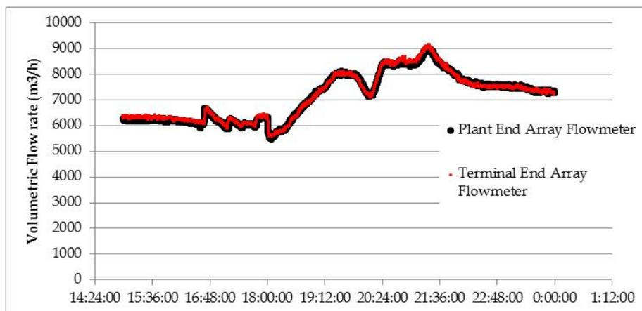
Figure 5. Volumetric flow readings at plant end and terminal ends using a SONARtrac array-based flow meter.
