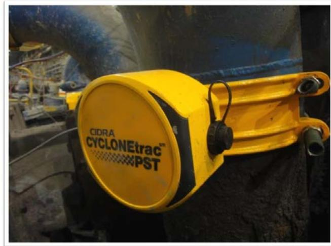
Figure 7. CYCLONetrac PST particle sizing sensor mounted on hydrocyclone overflow pipe.
