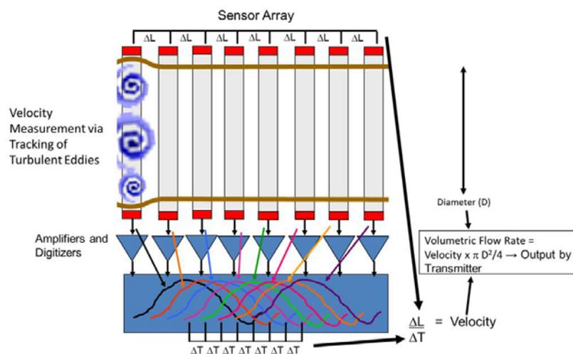
Figure 1. Illustration of signal detected by passive sensors in array from one collection of turbulent eddies.
