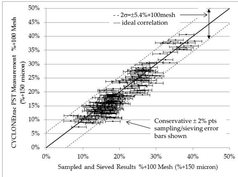
**Figure 4** CYCLONÉtrac PST 150 micron measurements compared to the sieved samples for a large copper concentrator
