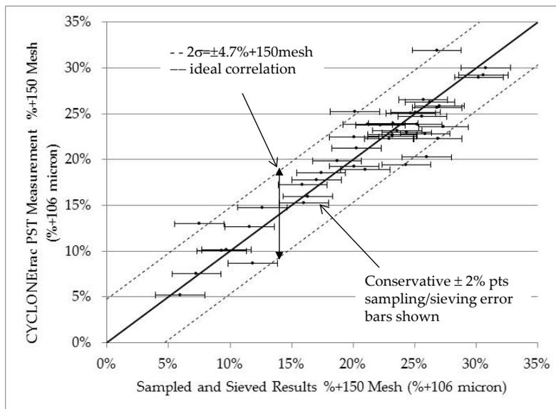
**Figure 5** CYCLONÉtrac PST 106 micron measurements compared to the sieved samples for a gold concentrator
