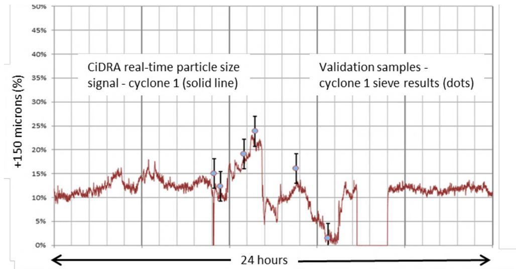
**Figure 13** Hydrocyclone 1 CiDRA CYCLONEtrac PST signal vs. validation sieve samples
