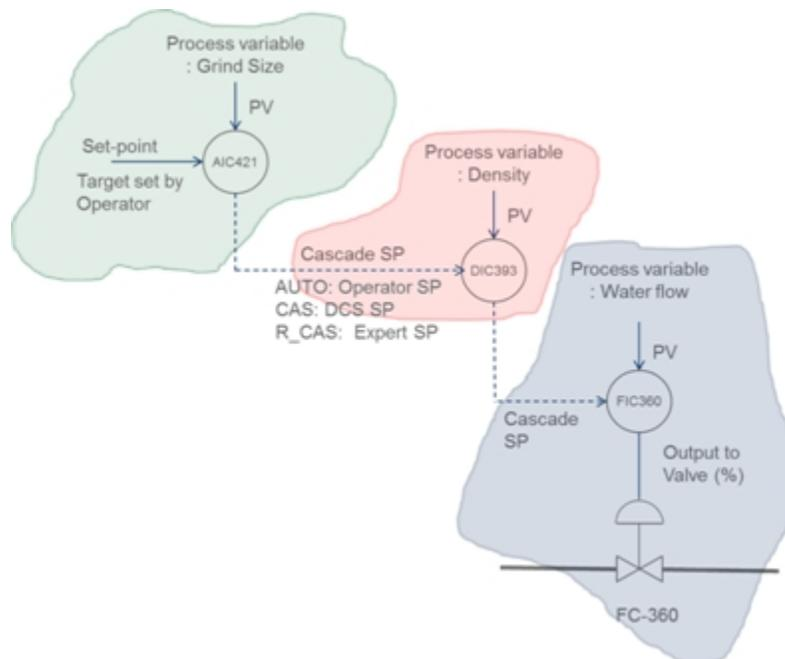
Figure 7 Cascaded control loops used to optimize grind value
