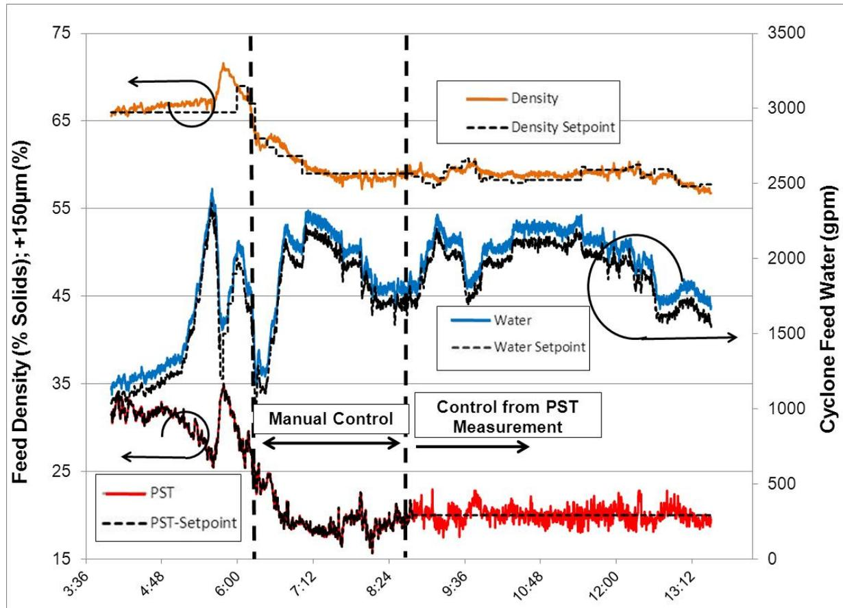
**Figure 8** Manipulating density for PST control
