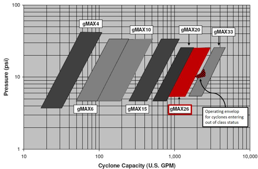
**Figure 10** FLSmidth Krebs gMAX capacity curves (FLSmidth)
