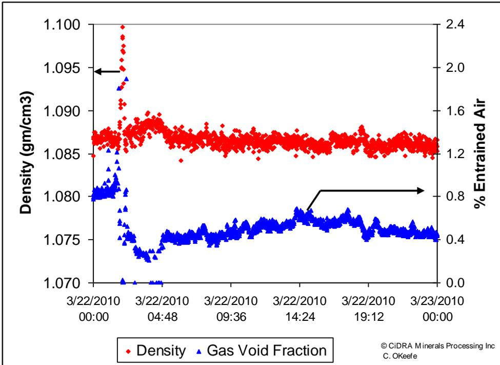
Figure 8 - Uncorrected density and Gas Void Fraction - 24 hour data set
