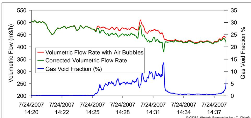
Figure 6 - Detection of entrained air bubbles and compensation of flow measurement
