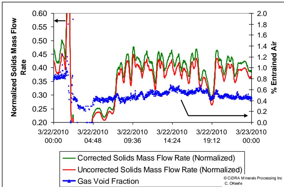
Figure 10 - Solids mass flow rate corrected for entrained air impact (green line) and uncorrected for entrained air (red line). Both have been normalized to an arbitrary mass flow rate.
