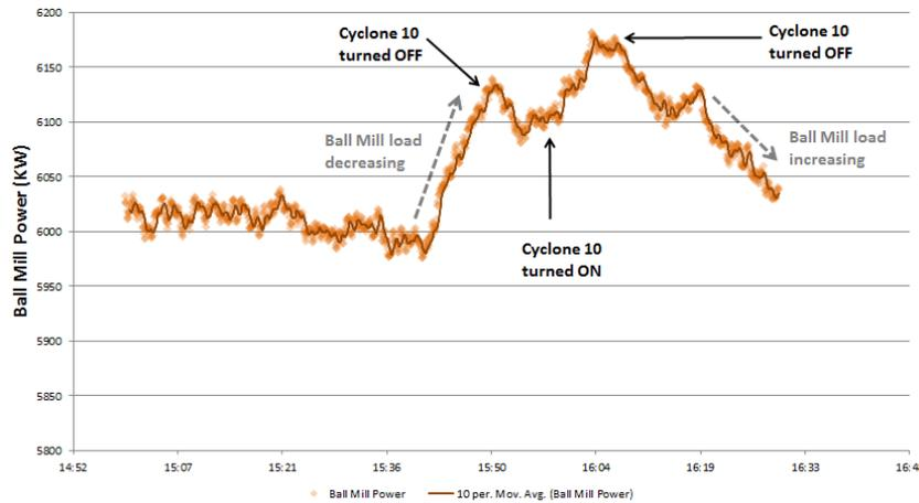
**Figure 7** Ball mill power over same 1.5 hour time period
