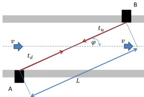
**Figure 1** Transit time flow meter operating principle
