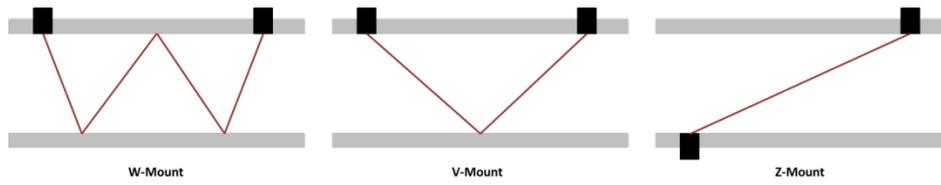
**Figure 2** Transceiver mounting configurations
