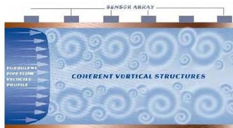
**Figure 5** Sensor array detecting coherent vortical structures convecting with the flow
