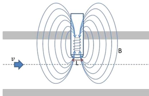
**Figure 6** Insertion mag meter measurement principle
