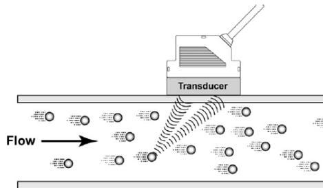
**Figure 3** Ultrasonic wave Doppler frequency shift
