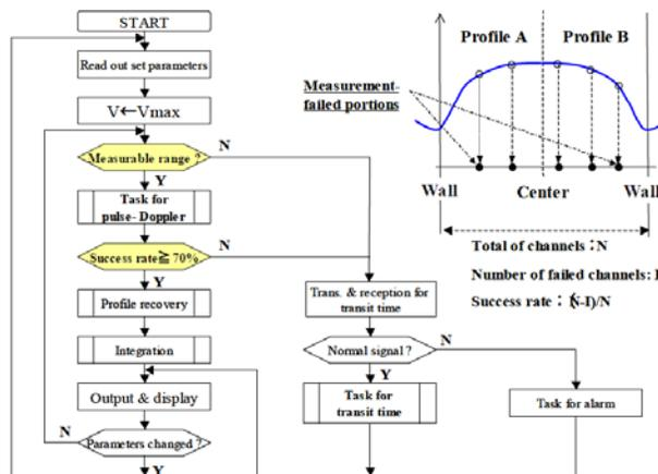
Figure 4 Hybrid ultrasonic flow meter switchover algorithm
