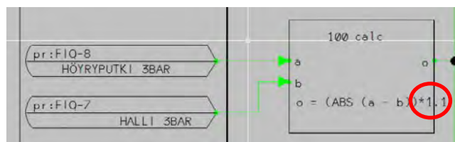
Figure 8 Old correction factor (1.1) was mistakenly left in signal calculation block in automation system.
