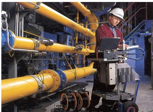
**Figure 5** On-site flow calibration on a natural gas line
