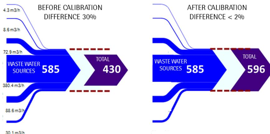
**Figure 6** Waste water balance before and after calibration of the total meter.
