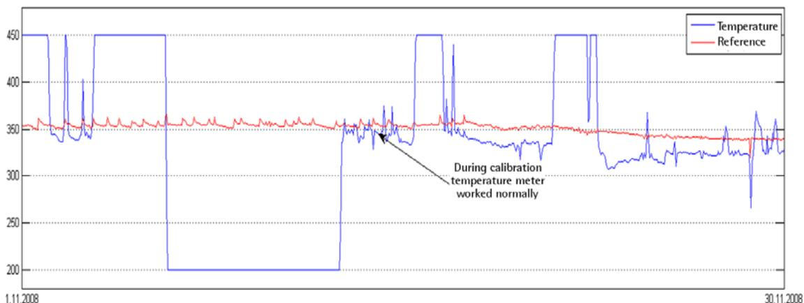
**Figure 9** The temperature signal used for density compensation of the flow meter was not operating properly.
