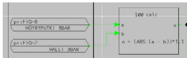
**Figure 8** An old correction factor (1.1) had been left by mistake to the signal calculation block in the automation system.
