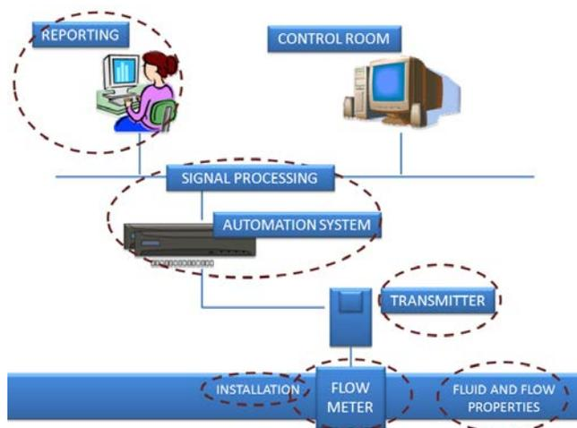
**Figure 3** Typically the biggest measurement errors are not caused by the meter itself, but arise from elsewhere in the measurement chain.
