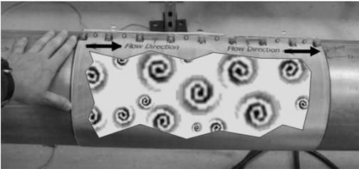
**Figure 1: Cutaway of Pipe Under Sonar Array Sensor Band to Illustrate Turbulent Eddies**
