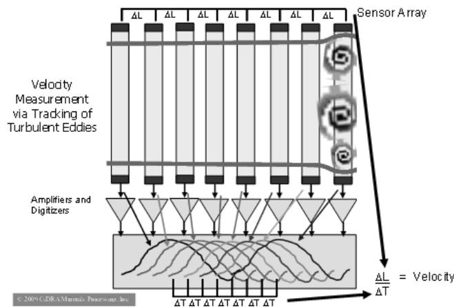
**Figure 2: Illustration of Velocity Measurement from Strain Induced in Pipe Walls by Passing Turbulent Eddies**
