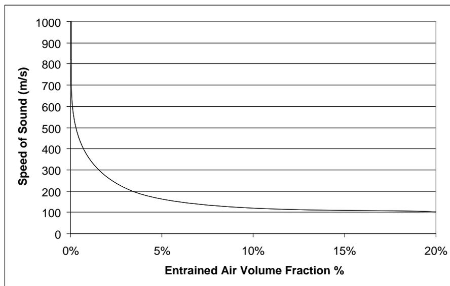
**Figure 4: Example of Relationship Between Speed of Sound and Entrained Air Volume Fraction (Gas Void Fraction)**
