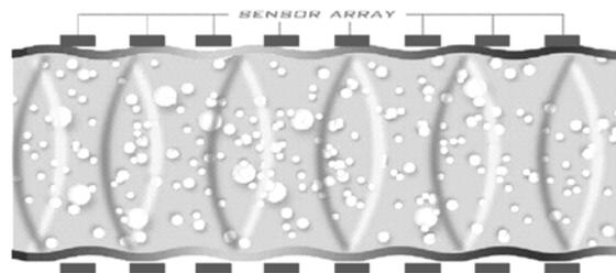
**Figure 3: Illustration of Naturally Occurring Acoustic Waves Propagating in Pipe Under the Array of Sensors**
