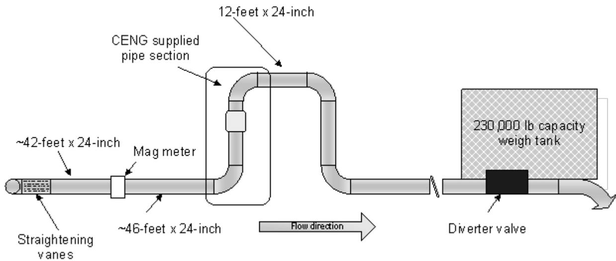
**Figure 8 Flow Loop Schematic**
