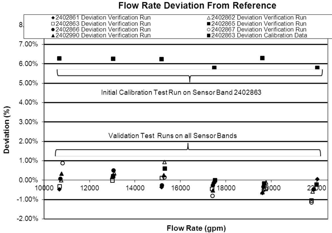
**Figure 10 Seven Sensor Bands Calibration Test Results**
