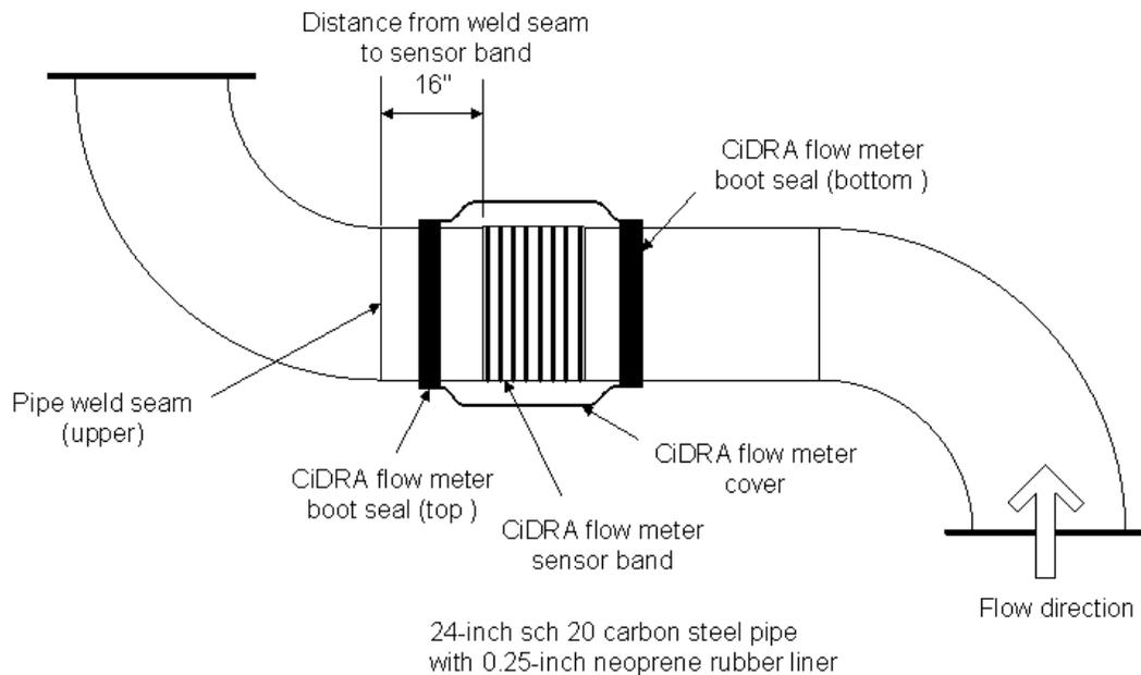
**Figure 9 Test Pipe Designed to be Identical to Installation Pipe**
