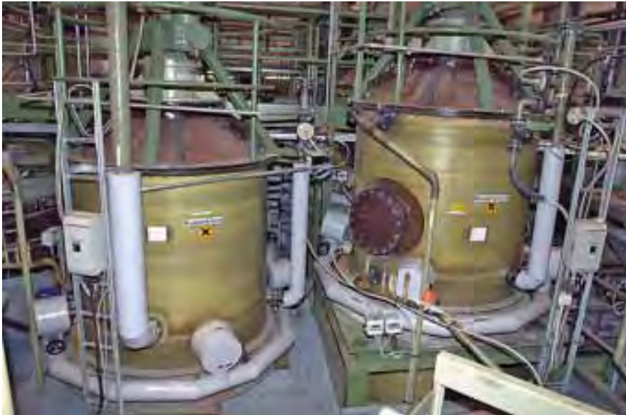
Outotec's HydroCopper® process produces high-quality copper wire rod directly from concentrates in a chloride environment. It is specially designed for chalcopyrite concentrates with unusual amounts of gold and silver. The product from the process is upcast copper rod and ready for further processing. HydroCopper consists of copper concentrate leaching, solution purification, and metal recovery by hydrogen reduction
