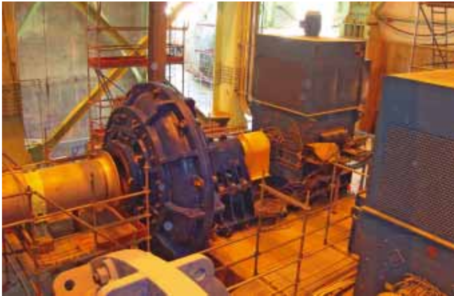
Warman says its rubber-lined MCR 750 is the largest mill circuit pump with moulded rubber liners in the world, and can be used in grinding circuits in large scale ferrous and non-ferrous mineral processing plants, such as copper. These pumps are currently being used at a copper mine in Chile
