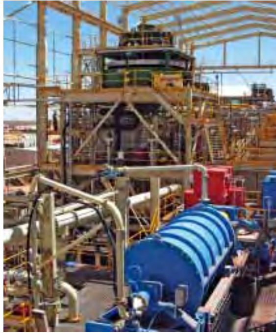
At Prominent Hill, a rougher concentrate is reduced from over 100µm to 24µm by a M10,000 IsaMill, and is then treated by a Jameson Cell
