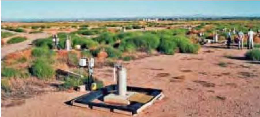
Injection well for ISCR
