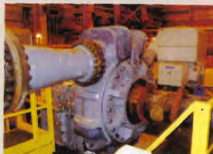
GIW centrifugal pump, Alberta oil sands
