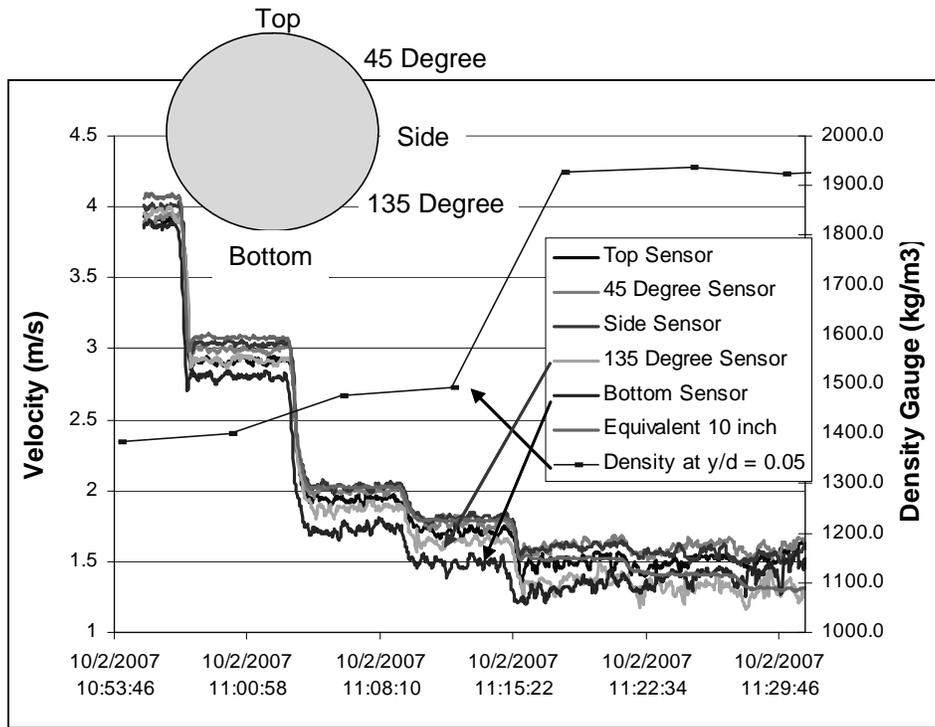
Figure 5: Velocity profile of 89  $\mu\text{m}$  mining slurry.
