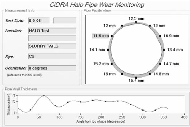
**Figure 18:** HALO™ pipe wall thickness visualization software output
