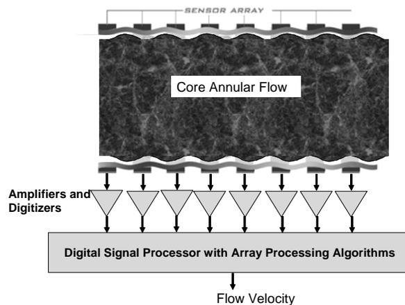
Figure 2 Diagram of pipe showing core annular flow with density variations and waves at core to annular interface
