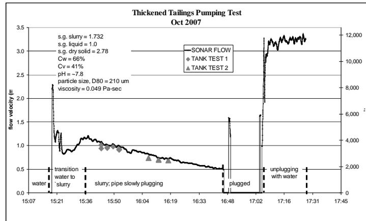
Figure 7 Thickened slurry test for Antofagasta Minerals, Chile, with flow measurements using sonar array-based flowmeter showing accuracy verified through tank fill tests and ability to operate at flow velocities below specifications.
