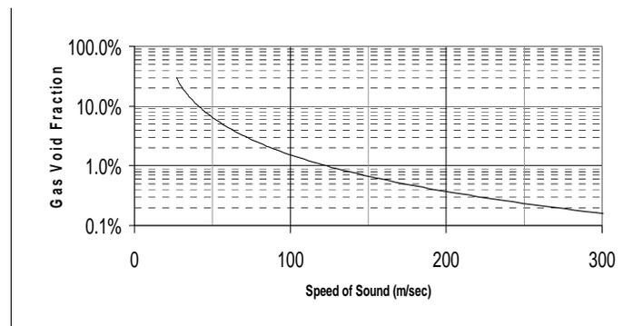
Figure 4 Example of relationship between gas void fraction (entrained air content) and speed of sound
