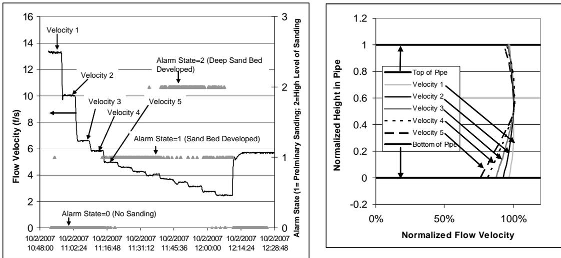
Figure 9 (Left) Normalized velocity profiles at various flow rates showing a drop in velocity at the bottom of the pipe at the lower flow rates. (Right) Flow velocity & alarm condition for low levels of sanding (Alarm level=1) and high levels of sanding (Alarm level=2)
