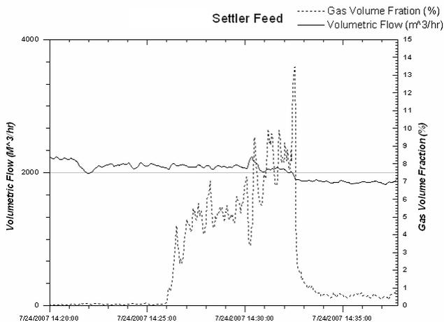
**Figure 15** Evidence of Flashing in Alumina Process
