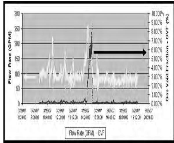
**Figure 14** Problems Measuring Both Flow and Gas Void Fraction in a Flotation Overflow Circuit is Solved. Effect on Pumping Efficiency and Resulting Drop in Flow Rate can now Determined by Measurement of Gas Void Fraction (Entrained Air)
