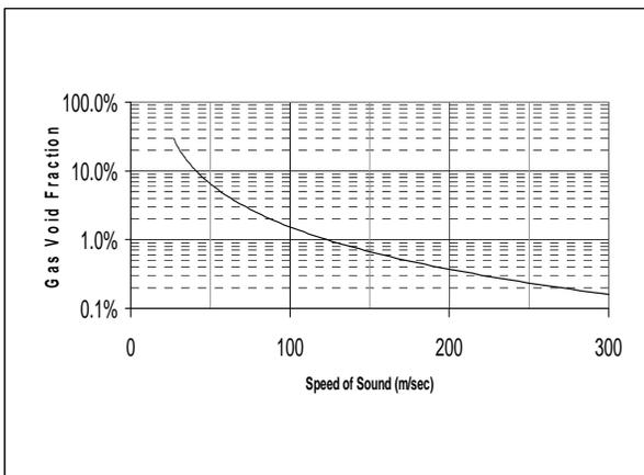
**Figure 2** Example of Relationship between Gas Void Fraction and Speed of Sound
