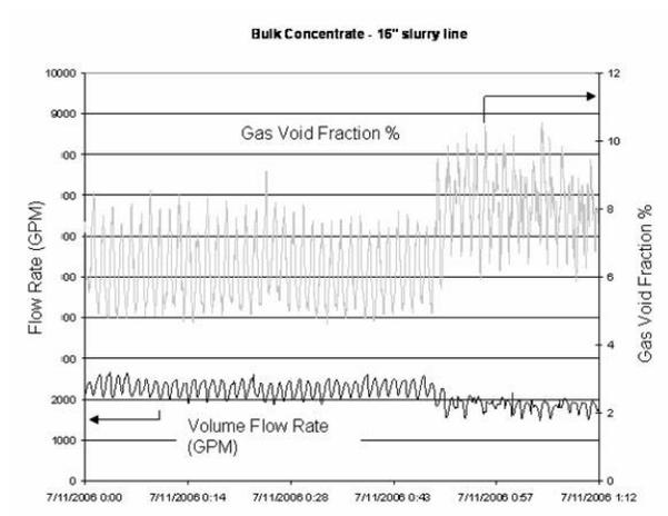
**Figure 12** Flow and Entrained Air (Gas Void Fraction%) Measurements Show Impact of Air on Flow Rate
