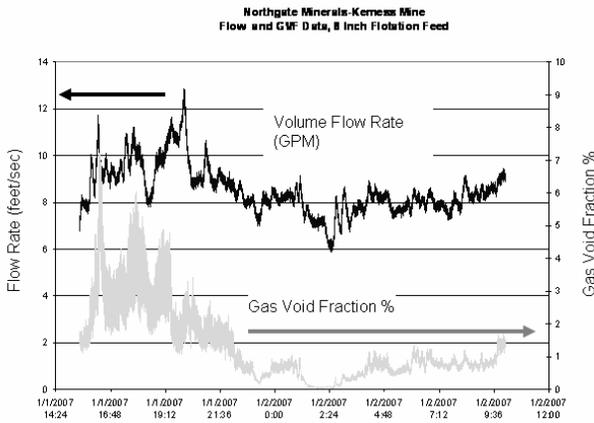
**Figure 13** Flotation Feed Line and Varying Air Levels Measured by Sonar Array-Based Instrumentation
