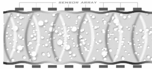
**Figure 1 Illustration of Naturally Occurring Acoustic Waves Propagating in Pipe under the Sonar Array Sensors**
