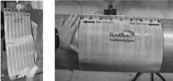
**Figure 6** Pictures of the Sensor Band with Drift-Free Sensor Elements
