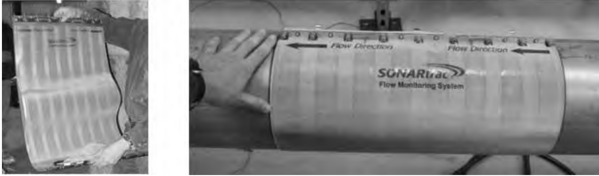
Figure 2 Pictures of the Sensor Band with Drift-Free Sensor Elements
