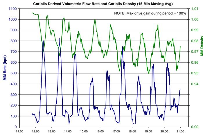
Figure 8: Coriolis Mass Flow and Density Reported During Well Test
