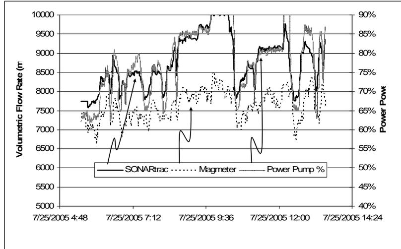
**Figure 13: Comparison of Sonar- Based Flowmeter with Magmeter and Pump Power Showing Excellent Correlation between Sonar- Based Flowmeter and Pump Power**
