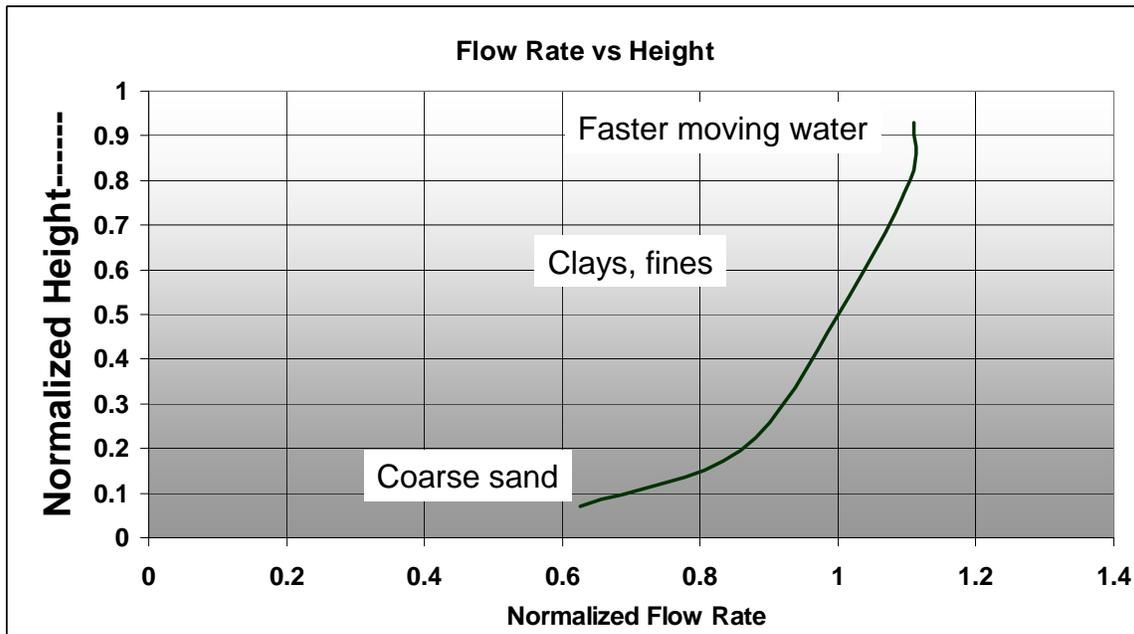
**Figure 16 Oil Sands Slurry Velocity Profile**
