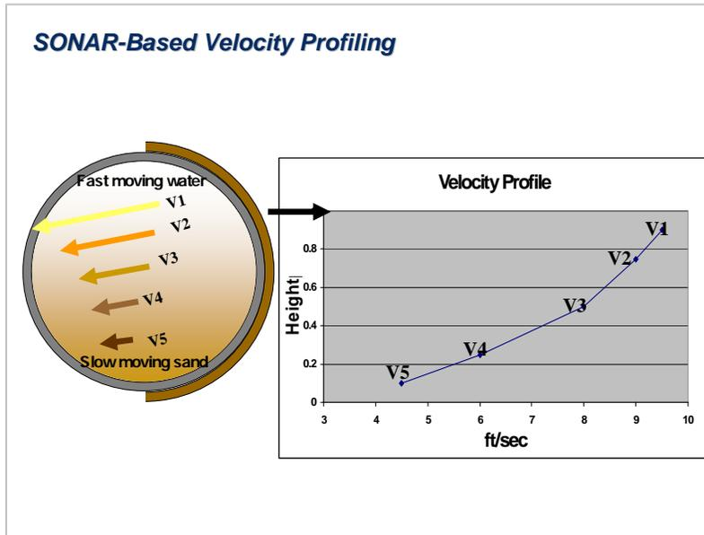
**Figure 15 SONAR-Based Velocity Profile**
