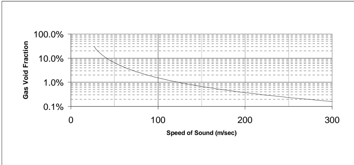
**Figure 8 Example of Relationship between Gas Void Fraction and Speed of Sound**
