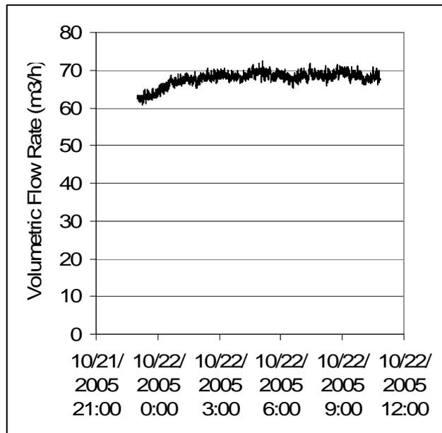
**Figure 15 Flow Reading in Magnetite Slurry**
