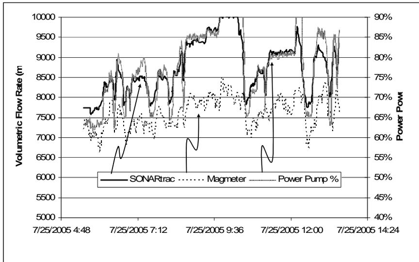
**Figure 9 Comparison of Sonar- Based Flowmeter with Magmeter and Pump Power Showing Excellent Correlation between Sonar- Based Flowmeter and Pump Power**
