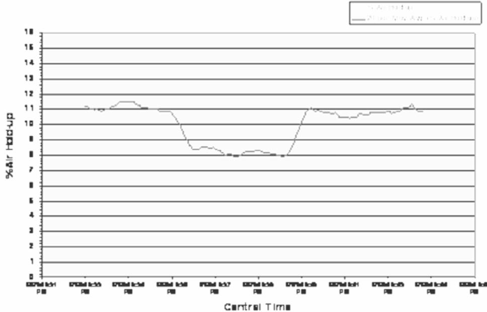
**Figure 21 Gas Holdup "Bump" Test in Copper Flotation Column (Y-Axis Range is 0% to 18% Gas Holdup)**
