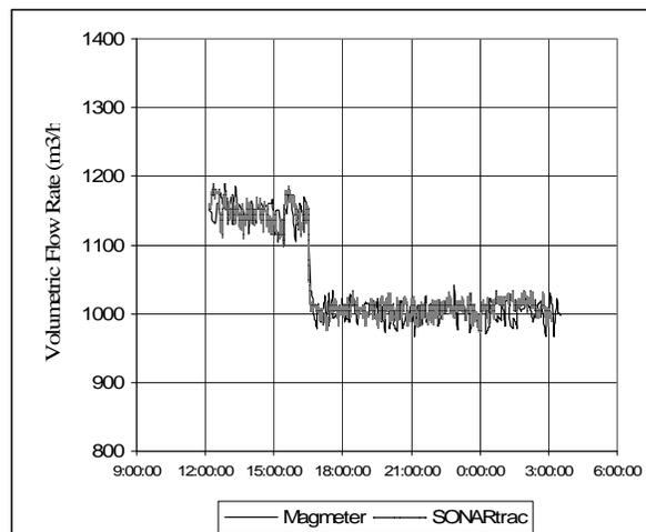
**Figure 11 Sonar- Based Flowmeter Operation in Water Pipe with Two Inches of Scale Buildup. Comparison to Recently Cleaned Magmeter is Shown.**
