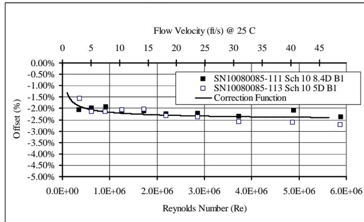
**Figure 3 Correction Required for a 10inch Schedule 40 Pipe**
