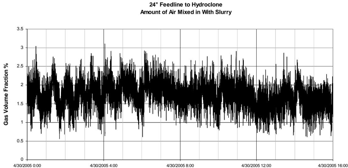
**Figure 17 Gas Void Fraction in a Hydrocyclone Feed Line**
