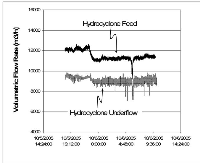
**Figure 10 Measurement of Flow in Hydrocyclone Feed and Overflow.**
