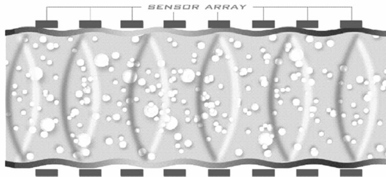
**Figure 6 Illustration of Naturally Occurring Acoustic Waves Propagating in Pipe under the Sonar Array Sensors**
