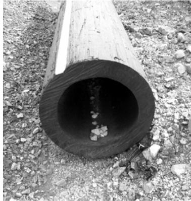
**Figure 13 Picture of HDPE Pipe Cross Section Showing a Typical Thick Wall**
