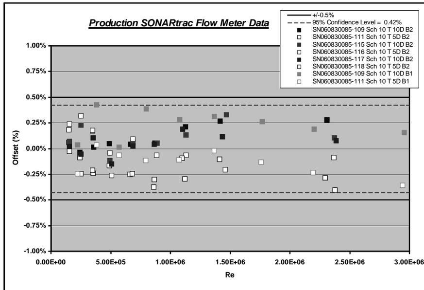
**Figure 5 Illustration of Calibration Consistency from Meter to Meter. All Meters Have Same Calibration Coefficients.**
