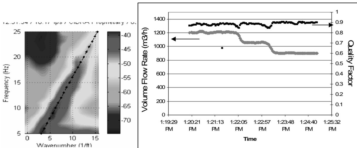
**Figure 12 (Left) Convective Ridge in  $K$ - $\omega$  Plot Showing Robust Measurement and (right) Flow Measurements Results with Good Volumetric Flow Measurement and Quality Factor**
