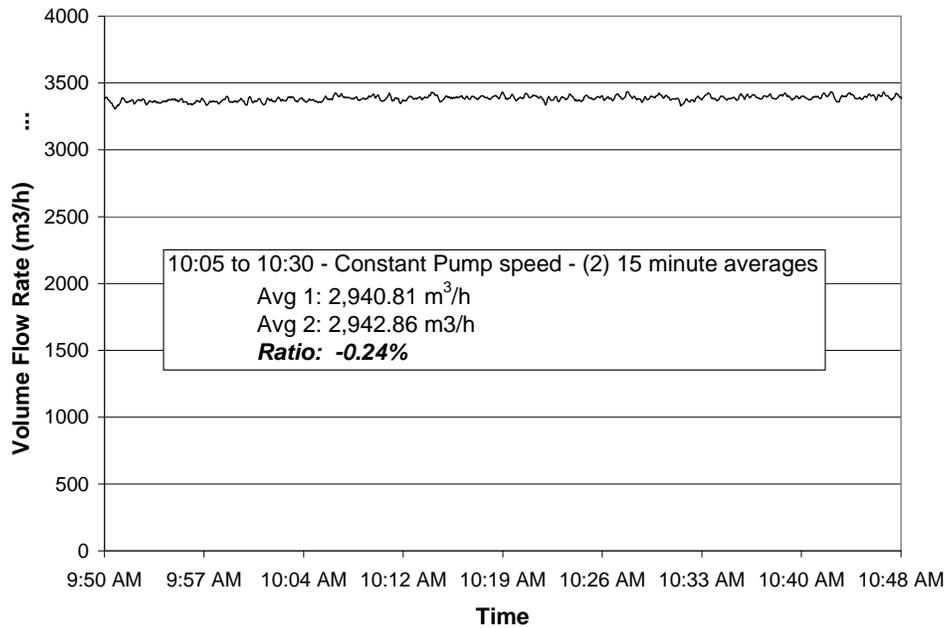
**Figure 16 Magnetite Tailings Line Noise Tests (At Least 20x Quieter than Magmeter)**
