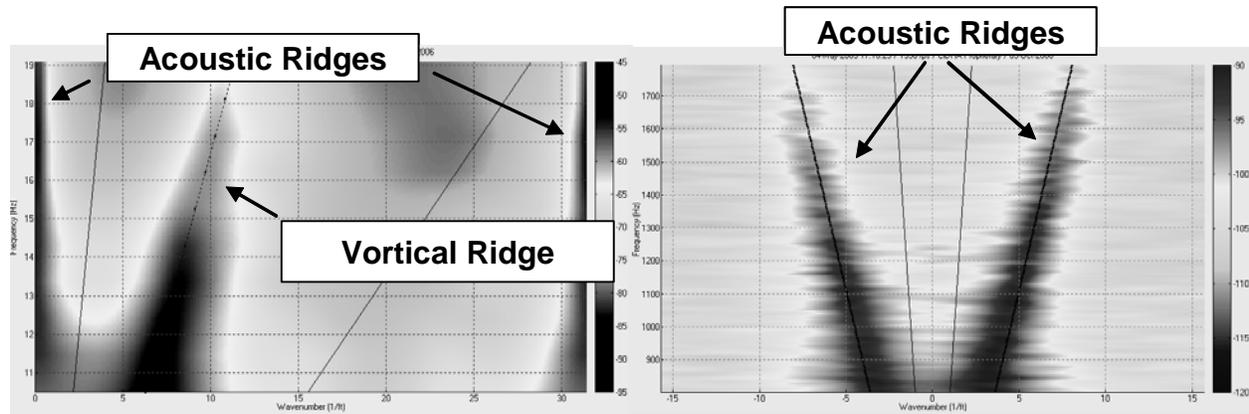
**Figure 7 (Left)  $k-\omega$  Plot Showing Both Acoustic Ridges and Vortical Ridge (Right) Rescaling of Graph and Change in Frequency Range Enhances View of Acoustic Ridges**
