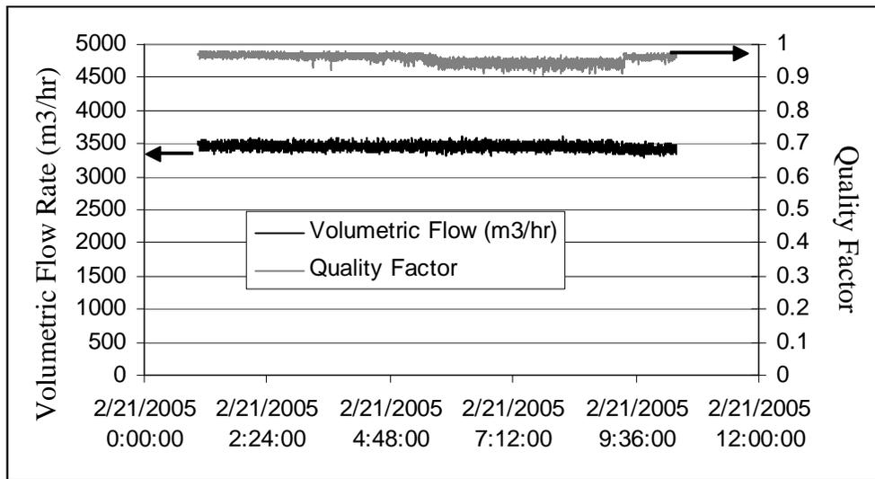
**Figure 14 Flow Measurements of Raffinate in a 30 inch High Density Polyethylene Pipe**
