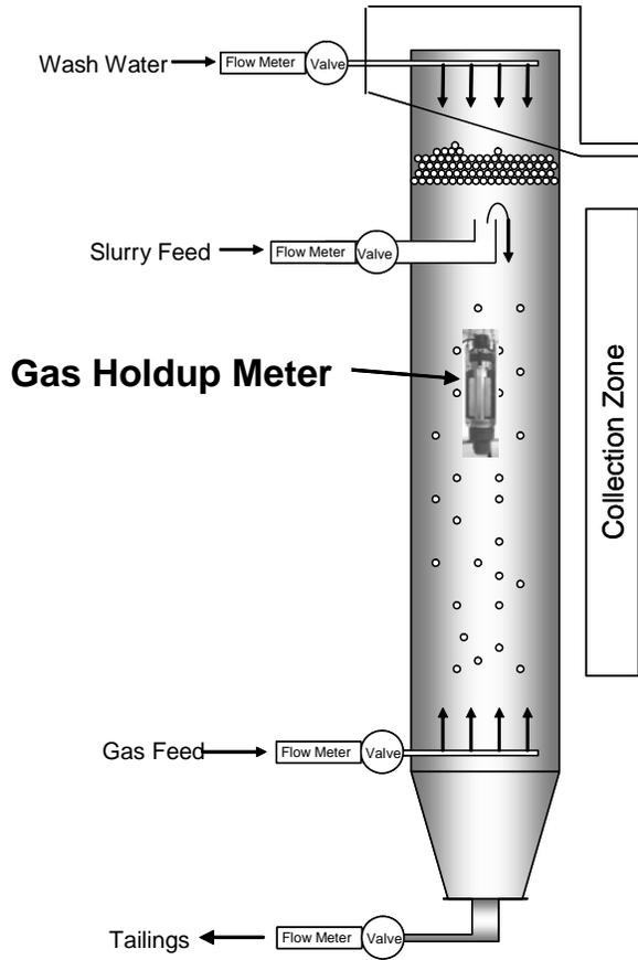
**Figure 20 (Left) Picture of Gas Holdup Meter and (Right) Diagram of Column Cell with Typical Location for Gas Holdup Meter**
