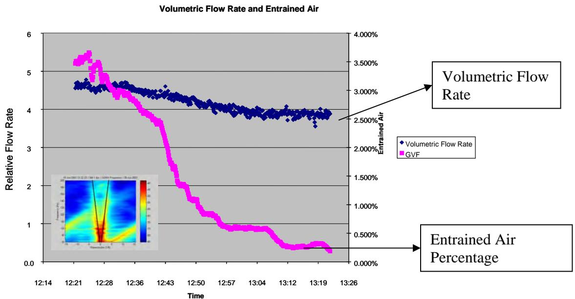
**Figure 19 SONARtrac Technology: Dual Measurements of Flow and Entrained Air Percentage (Gas Volume Fraction or GVF)**
