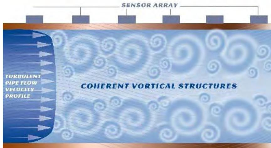
**Figure 1: Coherent Structures within Turbulent Pipe Flows**
