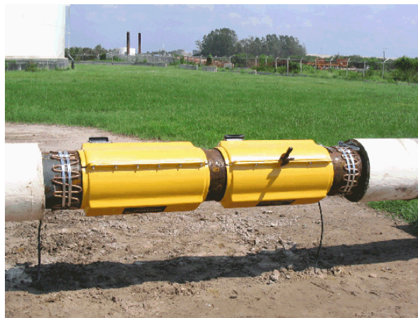
Sensor Heads With Insulation Removed and Ground Straps Installed
