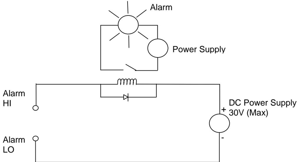
Figure 3 Example Alarm Circuit Diagram With Load Greater Than 100mA
