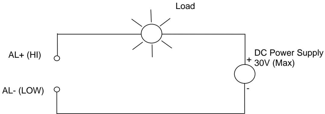
Figure 2 Example Alarm Circuit Diagram With Load 100mA Maximum
