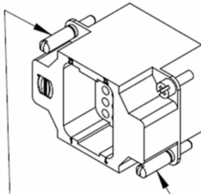
Figure 4 Guide Pin Installed in Base Assembly
