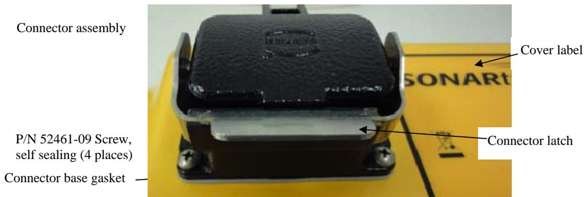
Figure 2 Connector Base Assy Gen-2 Cover (Outside Cover View)
