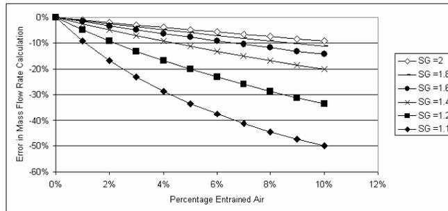
**Figure 15: Error introduced by entrained air in mass flow rate calculations as a function of slurry relative specific gravity (SG)**
