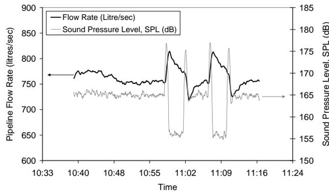
**Figure 18: Flow measurement and acoustic level measurement of a choke station while the valves are actuated.**
