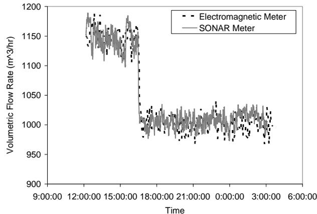
**Figure 16: Sonar array flowmeter operation on a water pipe with two inches of scale buildup compared to a recently cleaned electromagnetic flowmeter.**
