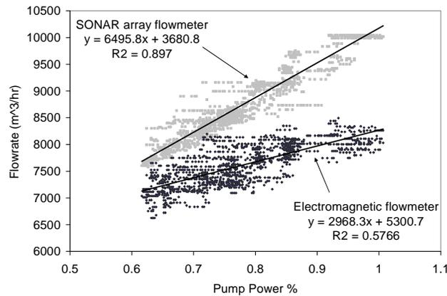
**Figure 9: Flow rate reported by sonar array based flowmeter and electromagnetic flowmeter relative to pump power (as percentage of maximum power)**
