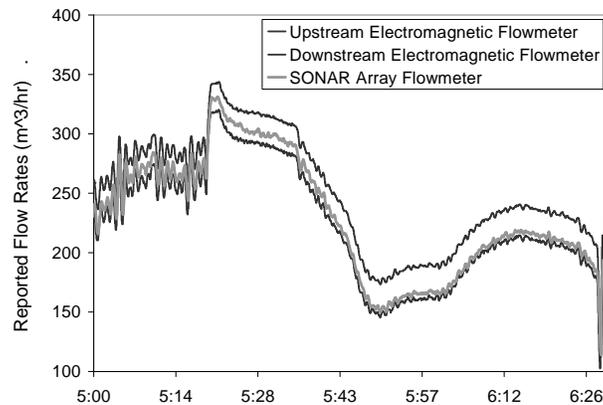
**Figure 6: Two electromagnetic flowmeters in series with sonar array flowmeter showing offsets greater than 12% between the two electromagnetic flowmeters and the drift of the electromagnetic flowmeters relative to the drift-free sonar array flowmeter**
