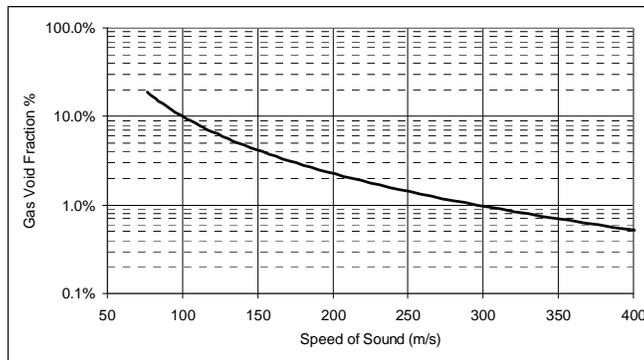
**Figure 4: Example of relationship between gas void fraction (entrained air bubbles) and speed of sound**
