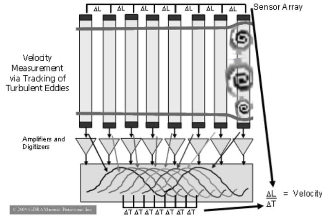
**Figure 2: Illustration of strain induced in pipe walls by passing turbulent eddies, resulting in similar signals detected by sensor elements with time or phase differences, leading to velocity measurement**
