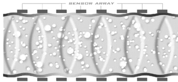
**Figure 3: Illustration of naturally occurring acoustic waves propagating in pipe under the array of sensors**
