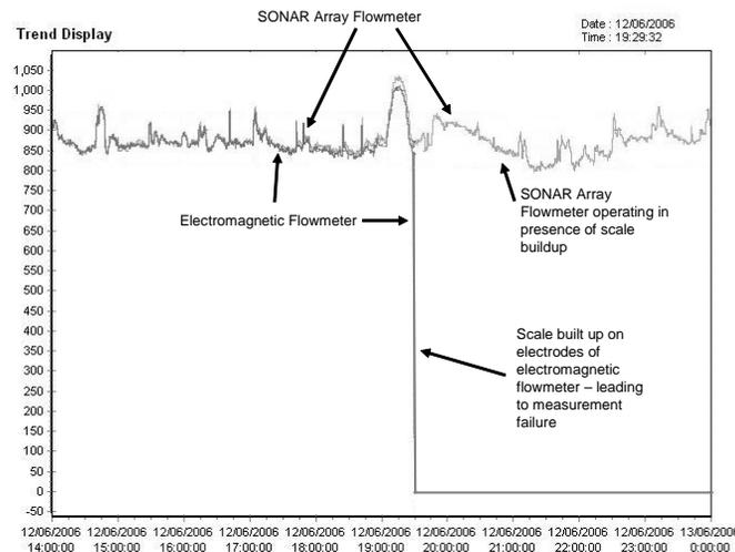
**Figure 17: Sonar flowmeter operation on a bauxite green liquor line with scale buildup during an electromagnetic meter failure.**
