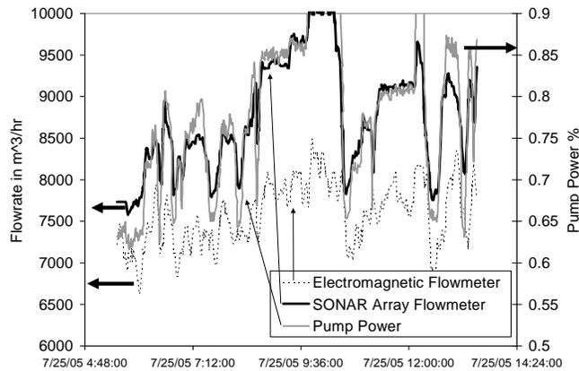
**Figure 8: Comparison of sonar array flowmeter and electromagnetic flowmeter to pump power on hydrocyclone feed line**
