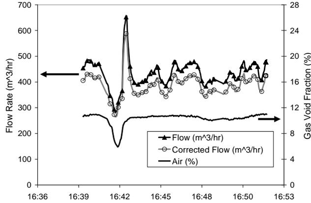
**Figure 13: Detection of entrained air bubbles and compensation of flow measurement**
