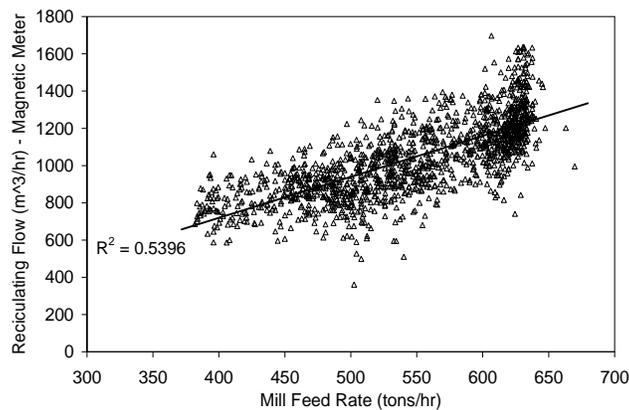
**Figure 10: Circulating flow rate versus mill feed rate as measured by the electromagnetic flowmeter.**
