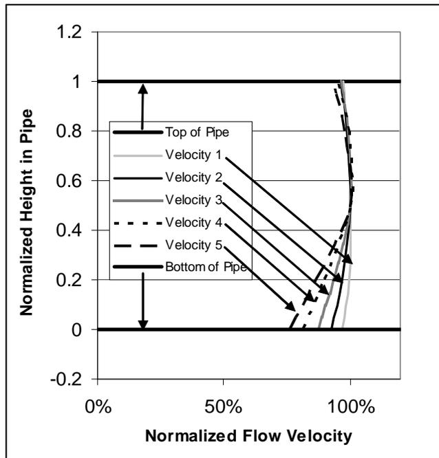
**Figure 20: Velocity profiles at different flow rates. Note the drop in velocity at the bottom of the pipe at the lower flow rates**
