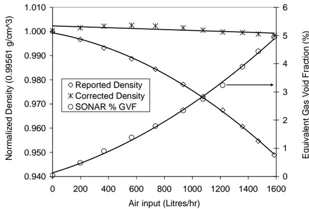
**Figure 14: Sonar array flow meter used to correct nuclear density gage for entrained air induced errors.**
