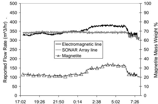
**Figure 12: Electromagnetic flowmeter erroneously respond to magnetite while sonar array flowmeter accurately reports flow**
