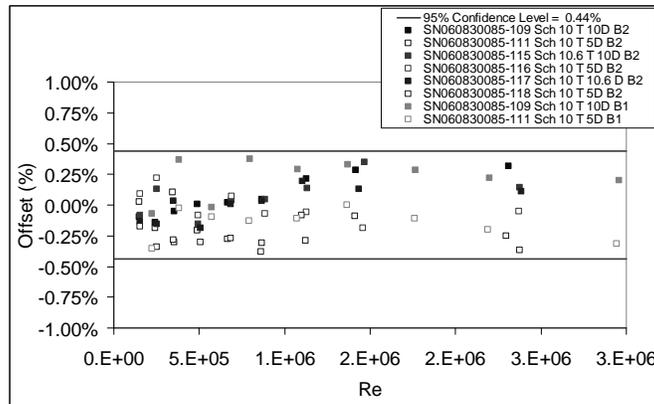
**Figure 7: Illustration of Calibration Consistency from Meter to Meter. All Meters Have Same Calibration Coefficients**
