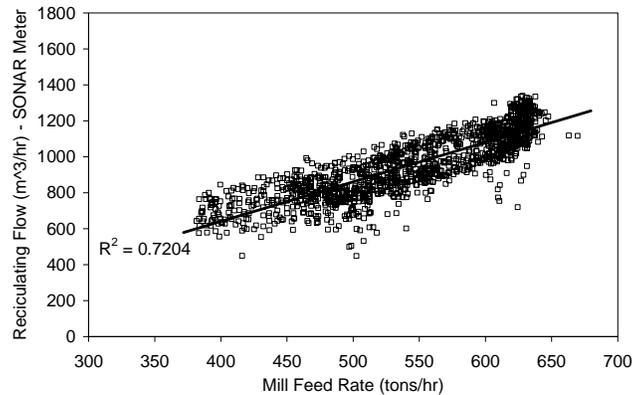
**Figure 11: Circulating flow rate versus mill feed rate as measured by the sonar array flowmeter.**
