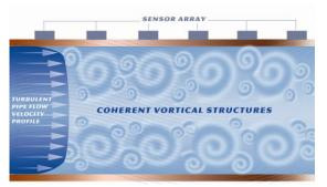
SONARtrac flow meters use a patented approach, based on well-established and mature sonar array processing techniques, to measure the velocity of these turbulent eddies as they convect past an array of sensors.
