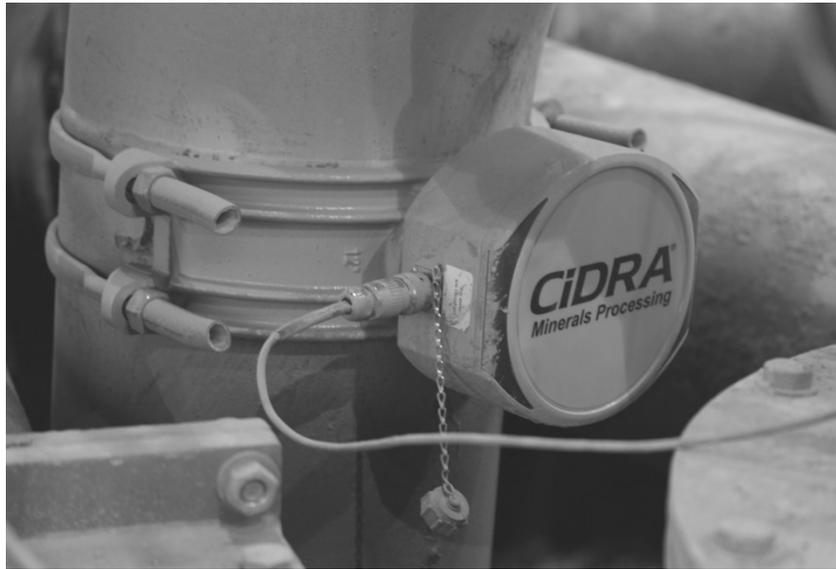
Figure 4: Sensor Head Assembly Mounted to Pipe
