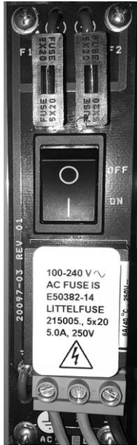
Figure 12: Mains Power Connection (NO POWER ENTRY BOX)
