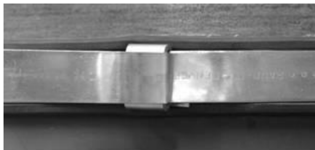
Figure 28 Band Clamp Final Installation
