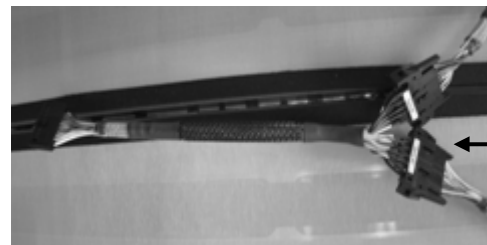
Figure 4 "Y" Connector Plugged into Sensor Band Connectors (P2 Upstream Band, P3 Downstream Band, P1 to Pre-Amp)
