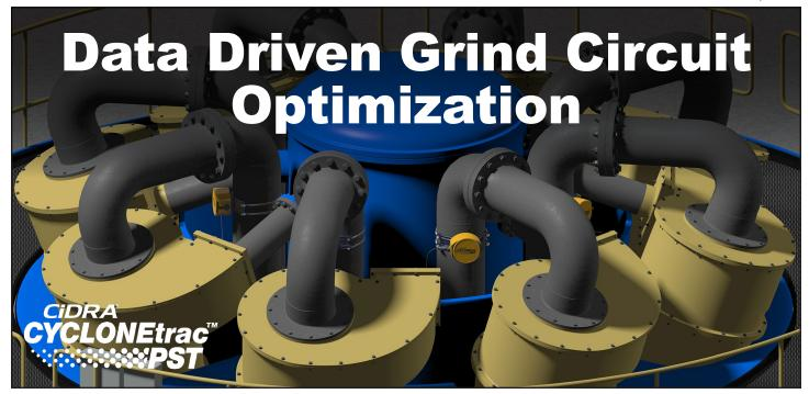
Hydrocyclone performance and particle size classification are crucial elements in the comminution process. The ability to measure particle size within individual cyclones is essential for grind circuit optimization and for controlling product size sent downstream.
