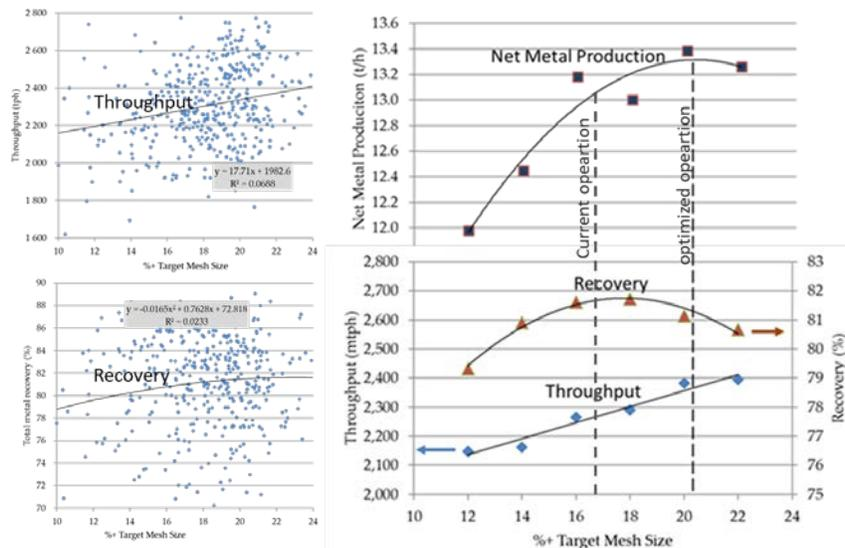
**Figure 5** Throughput & Recovery unfiltered (left), with data binning (right) with Net Metal Production (NMP) objective function per Equation 1.
