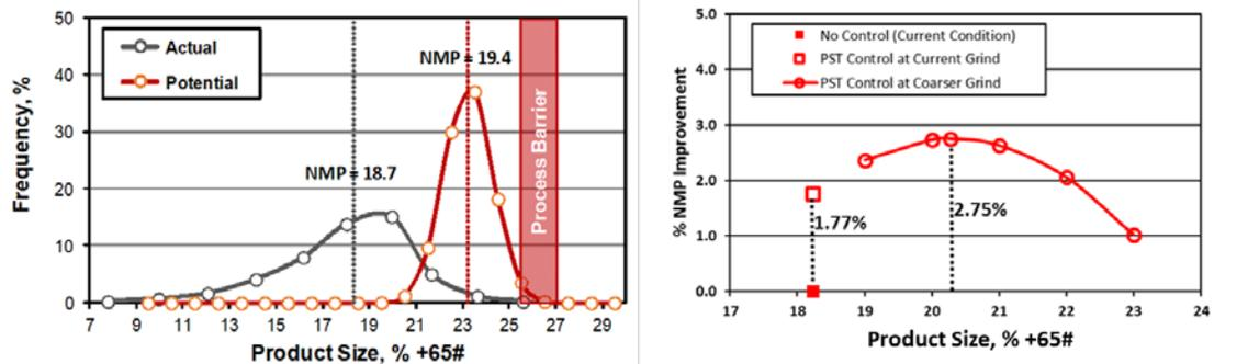
Figure 6 Actual and potential size distribution histograms and resultant NMPs (left), and associated potential percent NMP improvement (right).
