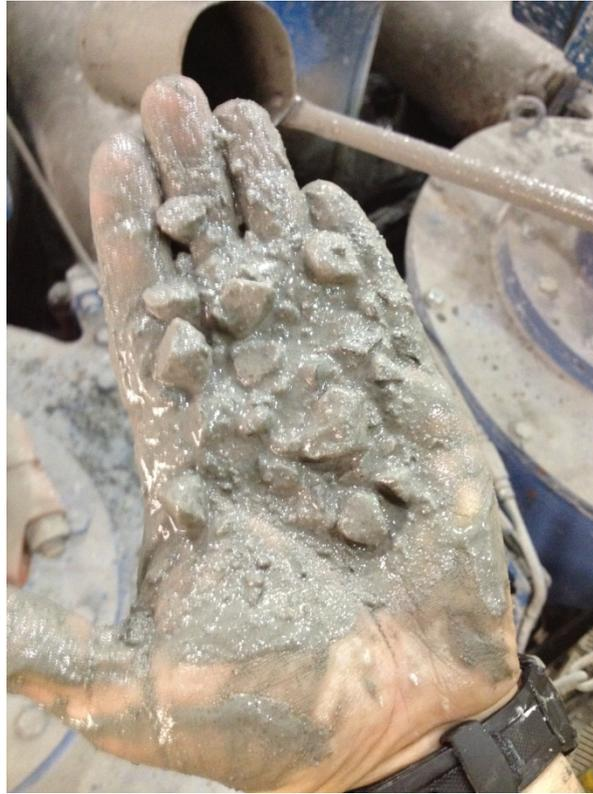
**Figure 6** During field validation, 78 samples were analyzed and compared to CYCLONetrac OSM pebble counts. Shown is an example of material collected during a pebbles/rocks event.
