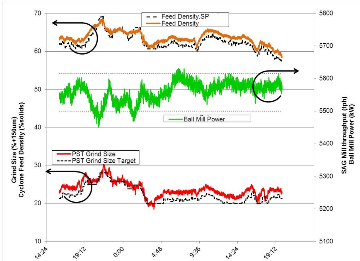
Figure 10 Example of particle size tracking leading to density setpoint changes and then to ball mill power draw
