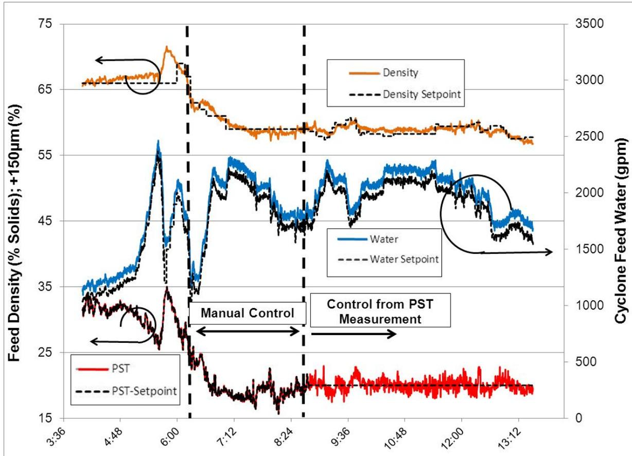
**Figure 8** Manipulating density for PST control
