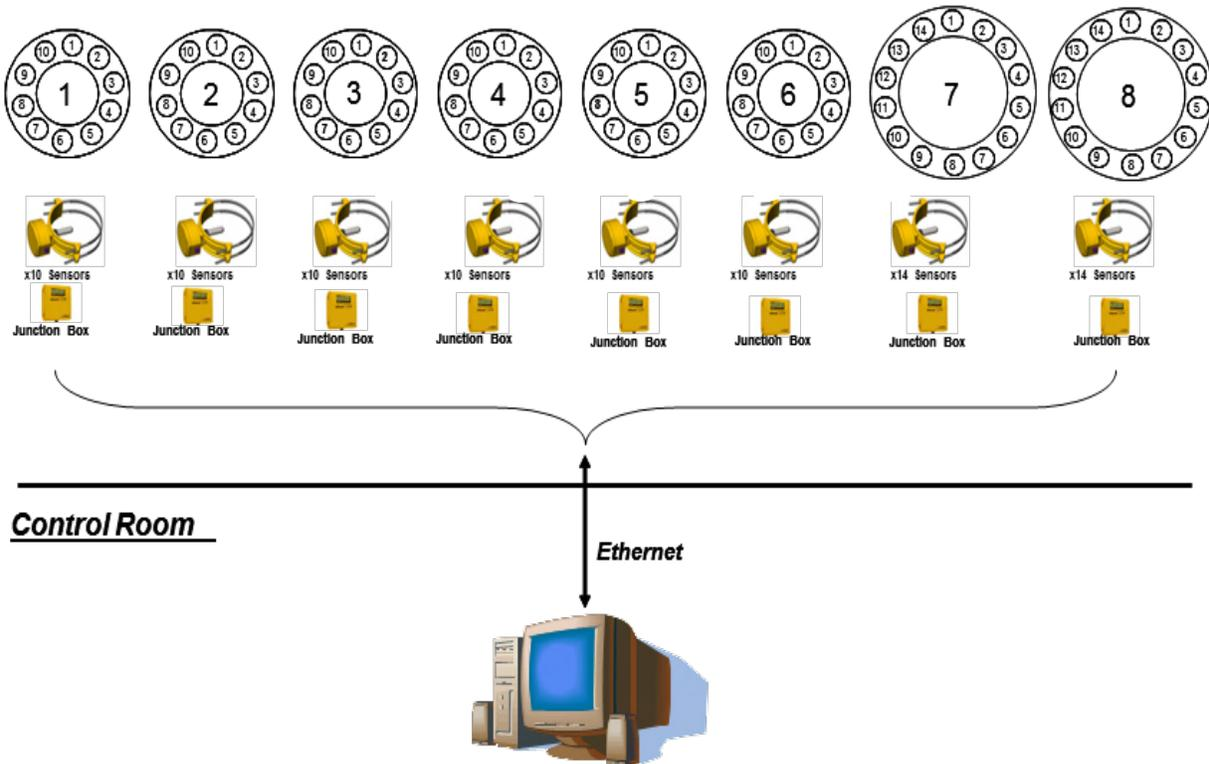
**Figure 12** Schematic of CYCLONetrac PST system installed at Rio Tinto Kennecott
