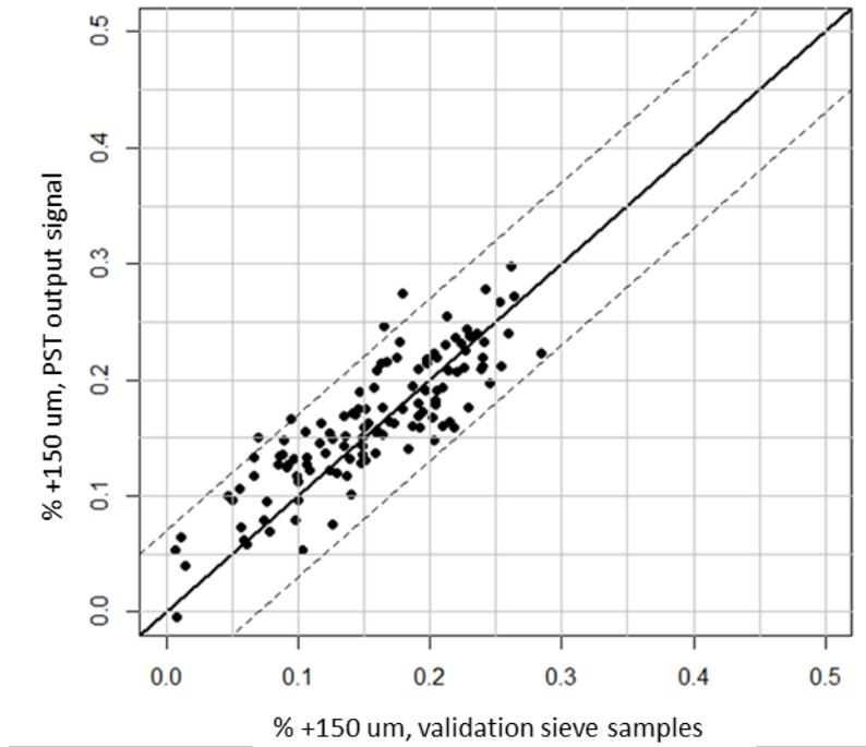
**Figure 14** Percent Mass Fraction +150 micron, CYCLONetrac PST output vs. validation sieve samples
