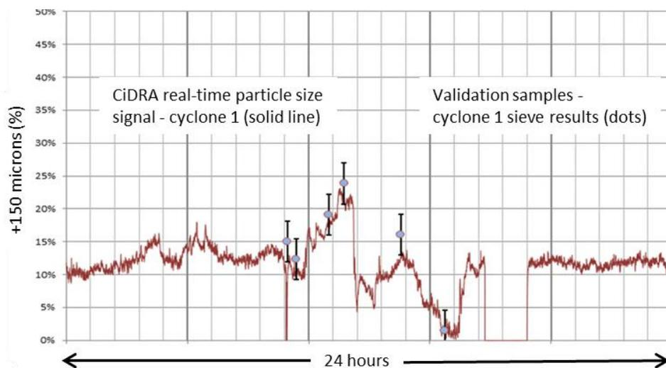
**Figure 7** Hydrocyclone 1 CiDRA CYCLONEtrac PST signal vs. validation sieve samples
