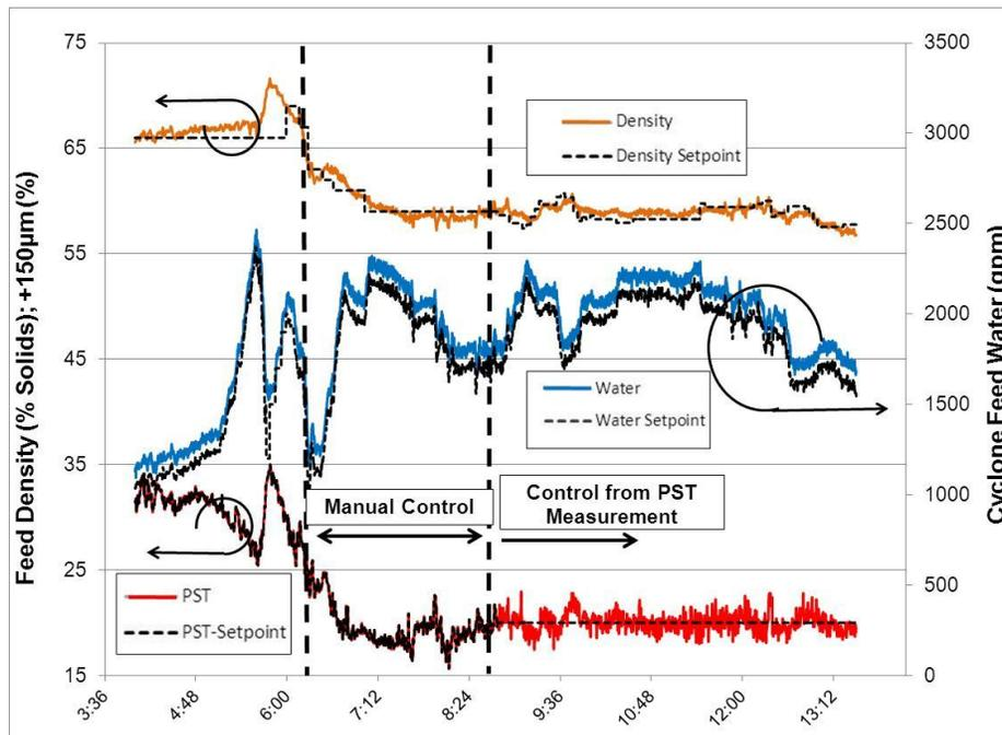
**Figure 2** Manipulating density for PST control
