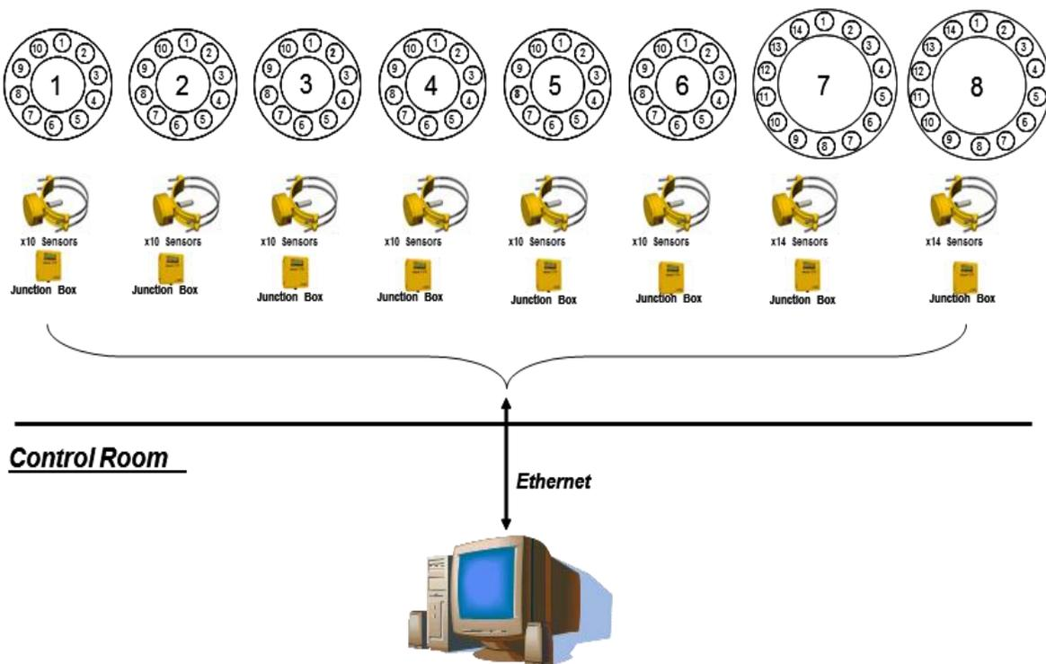
Figure 6 Schematic of CYCLONEtrac PST system installed at the Concentrator
