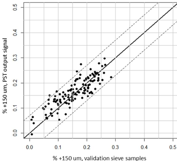
**Figure 8** Percent Mass Fraction +150 micron, CYCLONetrac PST output vs. validation sieve samples
