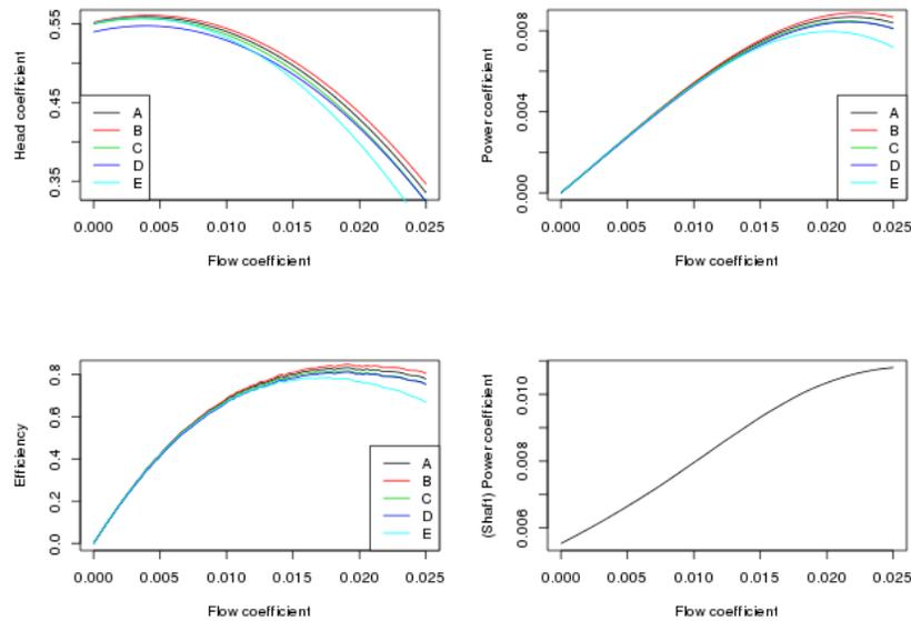
**Figure 2** Five pumps individually: three normal, two with issues
