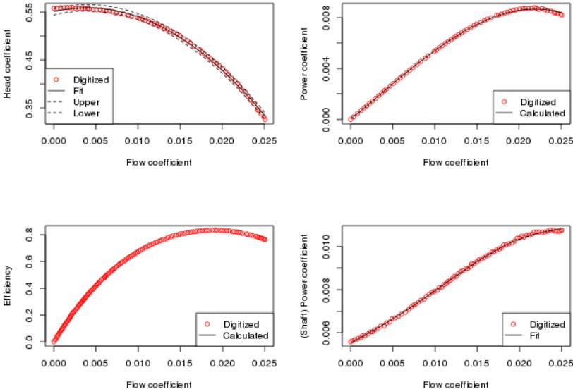
Figure 1 Digitized pump curve with best fit model
