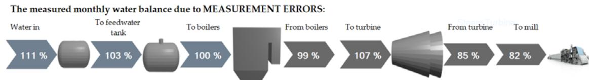
**Figure 2** The monthly water balance of a power production showing the effect of measurement errors. The recirculations and accumulations are taken into consideration so that all balance points should add up to 100%.
