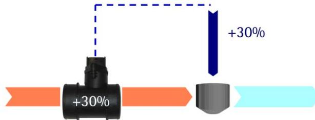
**Figure 1** Chemical dosage was 30% too high due to measurement error in waste water flow measurement
