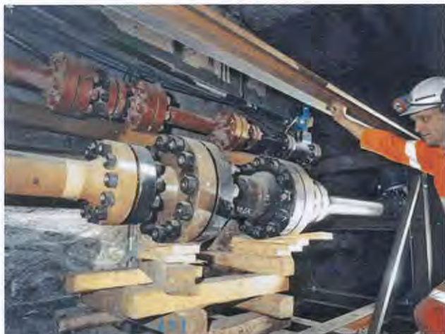
Paterson & Cooke's ED is a small unit which can dissipate hundreds of metres of head with a very compact footprint
