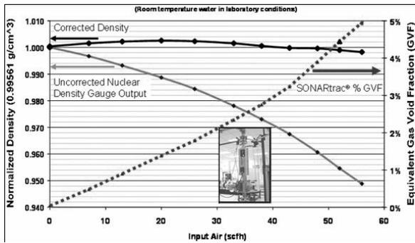
**Figure 10** Nuclear Density Gauge Correction using Sonar Array-Based flowmeter
