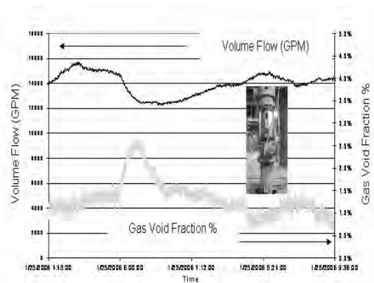
**Figure 9** Flow and Gas Void Fraction in a Hydrocyclone Feed Line
