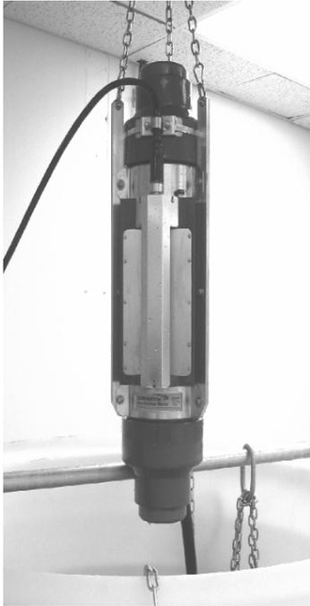
**Figure 5** Picture of Gas Holdup Meter Sensor Head for Submersible Application in Column Cells
