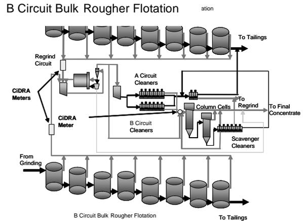
**Figure 11** Kemess Mills Flowsheet Showing Locations of Three Sonar Array-Based (CiDRA) Flowmeters
