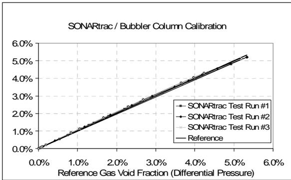
**Figure 8** Verification Test Results for Gas Void Fraction Meter on Calibration Column
